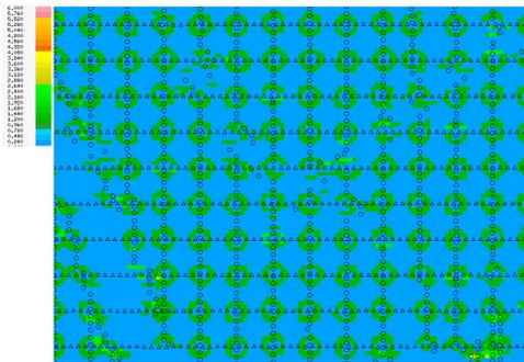
Figure 2 (a) Fold pattern at 150 m offset.
