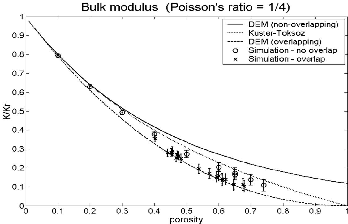
Figure 1. The dependence of bulk modulus on porosity. Theoretical results are shown by lines and simulation results by individual data points and error bars.
