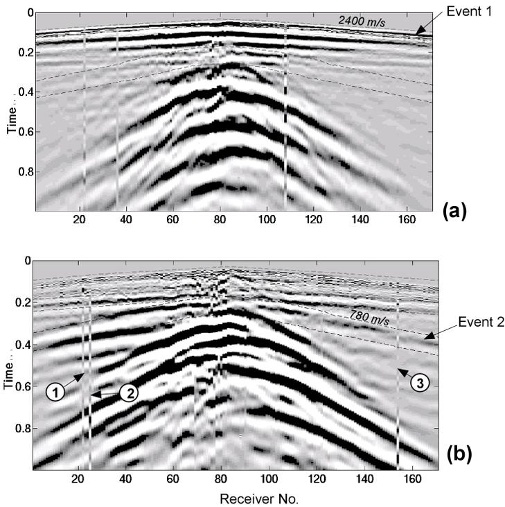
Figure 2. Seismic data set used.. (a) vertical component (b) horizontal in-line component. Windows corresponding to the events analyzed are illustrated. The numbers inside circles indicate reverse traces.
