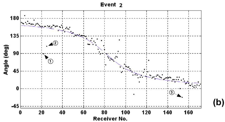
Figure 5. Covariance matrix analysis of the two events. (a) First breaks – P-wave refractions (b) S-wave refraction. Numbers inside circles correspond to reverse traces in Fig. 2.
