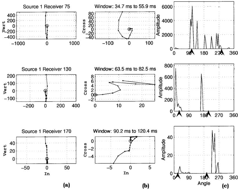
Figure 3. Hodogram and histogram analysis of the first event (P-refraction). (a) Side hodogram (b) top hodogram (c) histogram. Arrows indicate angles from field geometry.
