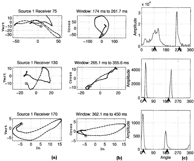
Figure 4. Hodogram and histogram analysis of the second event. (S-refraction). (a) Side hodogram (b) top hodogram (c) histogram. Arrows indicate angles from field geometry.
