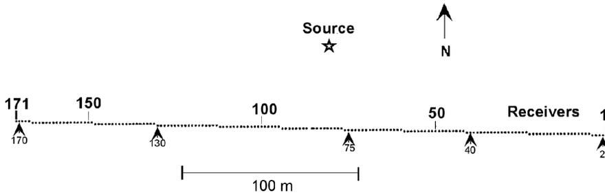
Figure 1. Geophone layout and source location used for the experiment.
