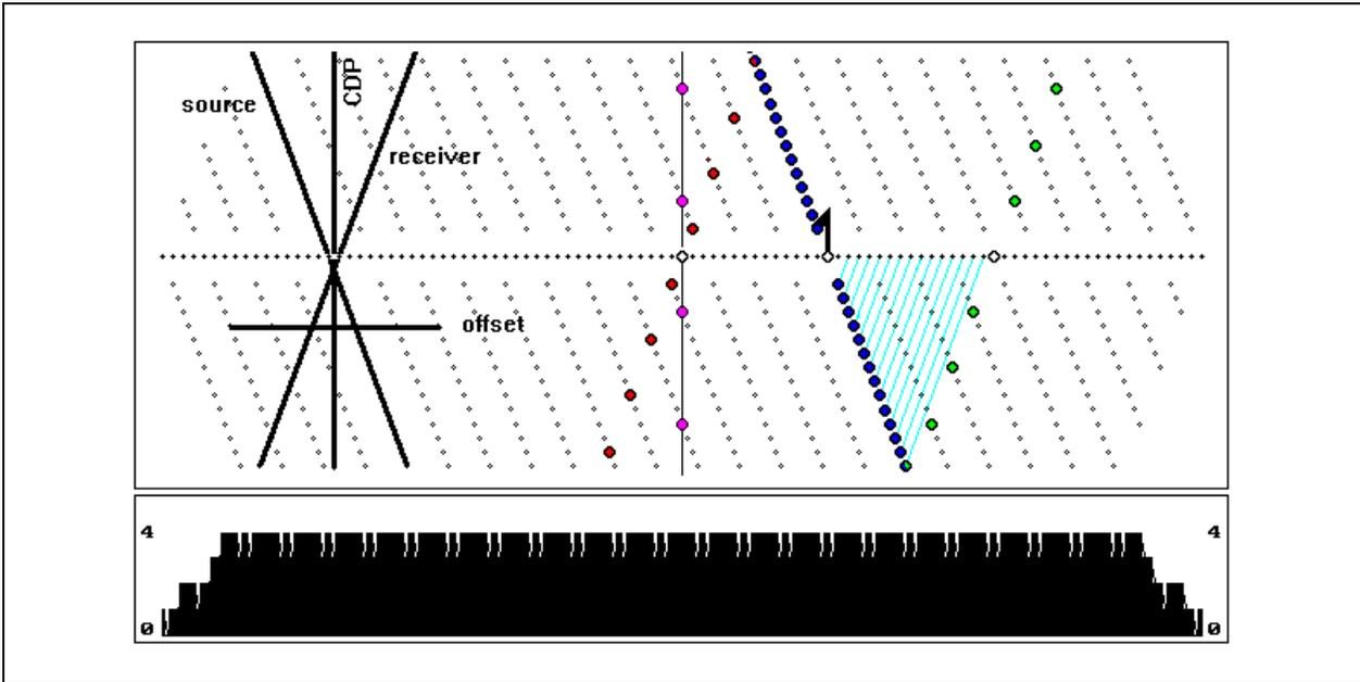
**Figure 2** A portion of a 2D stacking chart for a line with a receiver interval of 20 meters and a source interval of 80 meters. The sources were located coincident with receiver points
