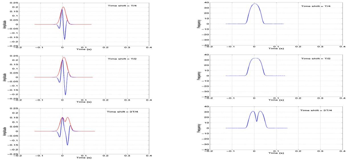
Figure 1 Interfering opposite-polarity Ricker wavelets spaced by  $T/4$ ,  $T/2$  and  $3T/4$  ( $1/T$  is the dominant frequency, 30 Hz) and the respective diagrams of instantaneous amplitude (left, red) and frequency (right, blue).
