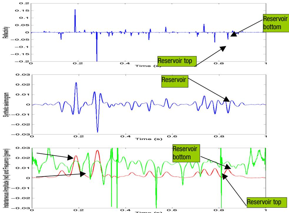
Figure 2 Upper: random reflectivity series generated from Matlab command `Reflect(1, 0.002)`; Middle: synthetic seismogram generated from convolution of the random reflectivity series( Figure1) with the Ricker wavelet (30Hz); Lower: instantaneous amplitude (red) and instantaneous frequency (green, \*2000).
