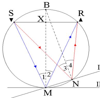
Figure 1: Incident angles for the horizontal and dipping reflectors with source S and receiver R.
