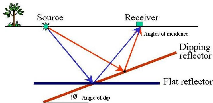
Figure 3: Orientation of source, receiver, and reflector for modeling study.
