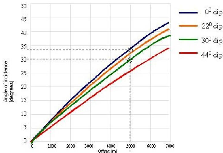
Figure 4: Actual angles of incidence vs. offset for reflection from top of dipping layer, for dips of  $0^\circ$ ,  $22^\circ$ ,  $30^\circ$  and  $44^\circ$ .
