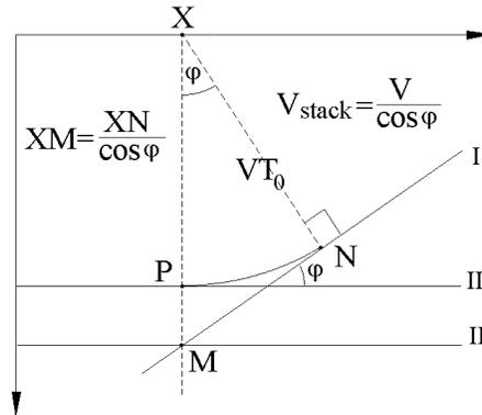
Figure 2: Dipping boundary I and its equivalent II:  $XM = V_{\text{stack}} T_0$ ,  $XP = XN = V T_0$
