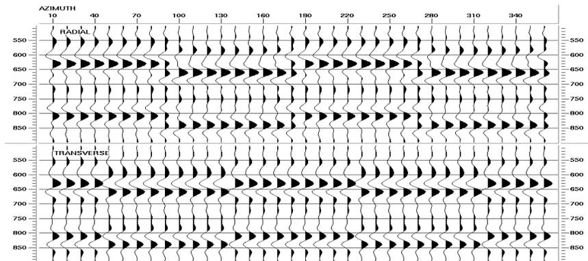
Figure 8: Limited-azimuth stacks for a single anisotropic layer with an  $S_1$  azimuth of  $45^\circ$  and a time delay of 30 ms.
