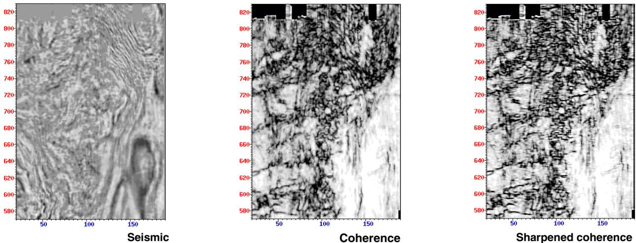
FIGURE 1: Coherence slice not only shows up faults with clarity but also the intensively fractured region to the top
