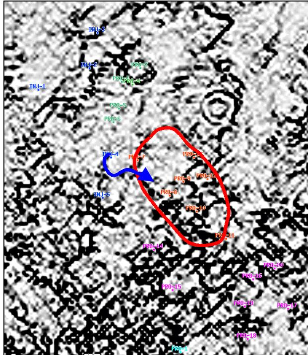
FIGURE 5: Horizon slices from coherence volume 68 ms below the horizon representing the reservoir top. Wells inside red area had one (1) day to breakthrough.
