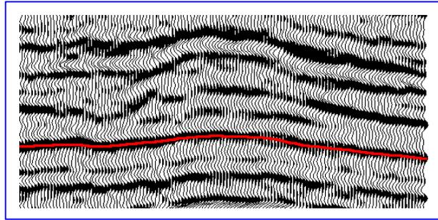
Segment of seismic line after high frequency restoration showing the reef
