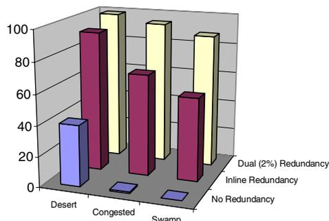
Figure 5 Projected availability with different redundancy
