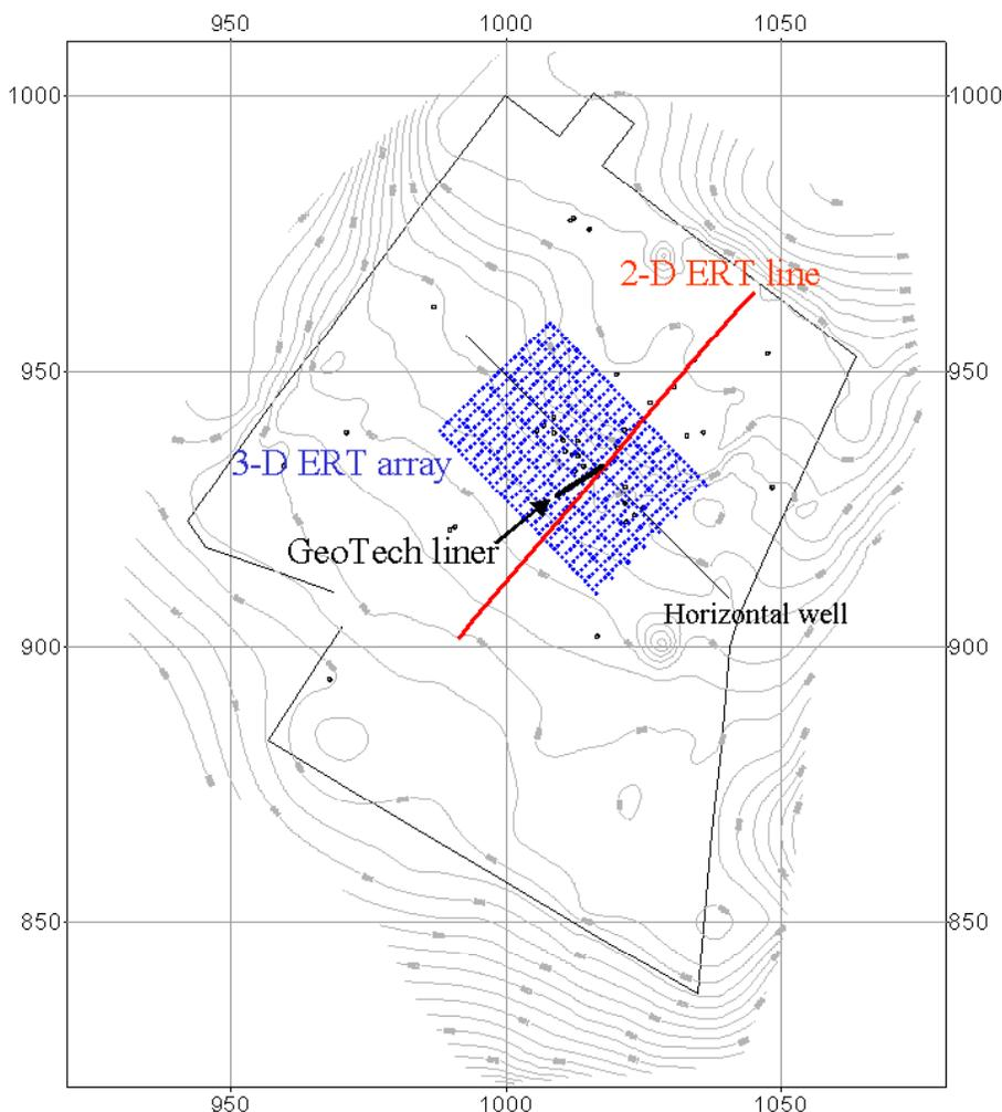
Figure 1. Location map. Blue plus symbols show the location of current and potential electrodes in 3-D ERT array.
