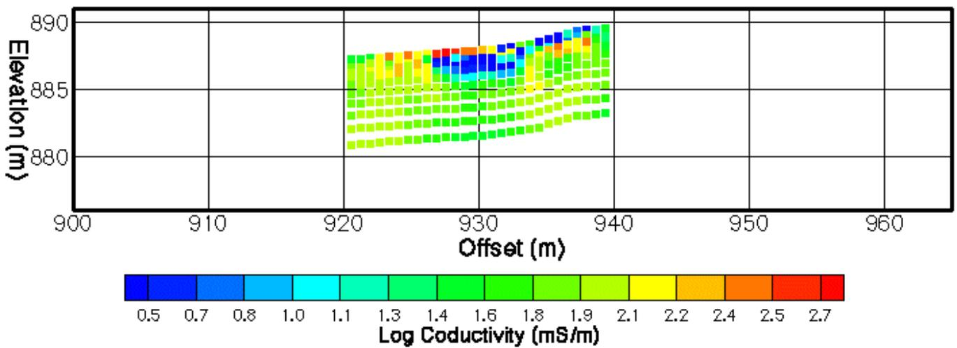
Figure 4. 2-D conductivity section after inversion of 3-D ERT data. The section coincides the 2-D ERT line where it parallels 3-D ERT array.
