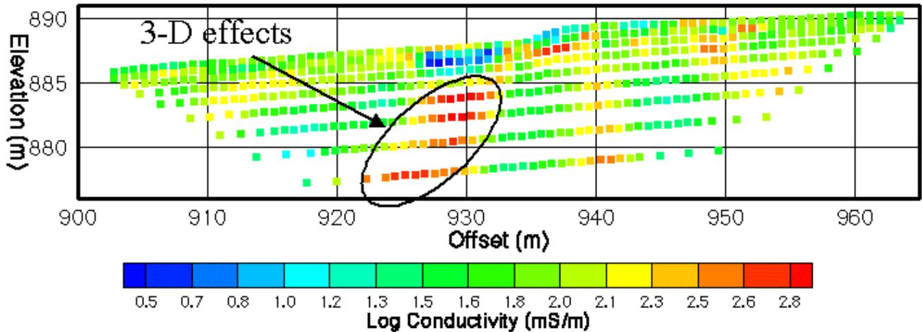
Figure 2. Conductivity section after inversion of 2-D ERT line.
