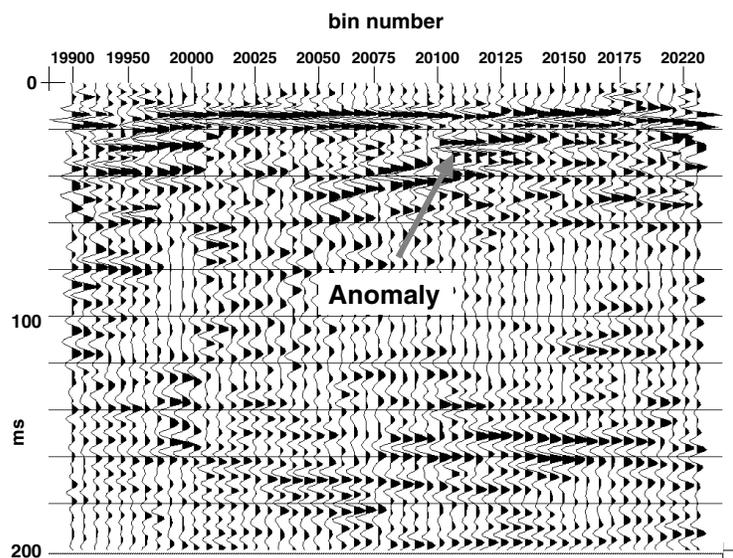
Figure 1. P-P reflection image formed from vertical component of 2000 Chan Chich 3-C seismic survey. Length of the survey is 20m
