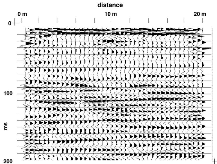
Figure 3. P-P reflection image formed from vertical component of 2001 Chan Chich 3-C seismic survey.
