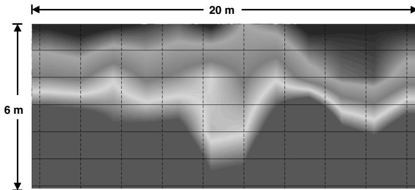
**Turning-ray tomographic image of near surface at Chan Chich, from first breaks**
