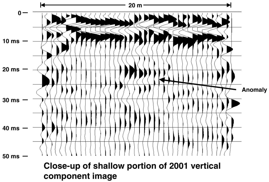
Figure 6. Close-up of P-P reflection section formed from vertical component of the 2001 Chan Chich 3-C seismic survey.
