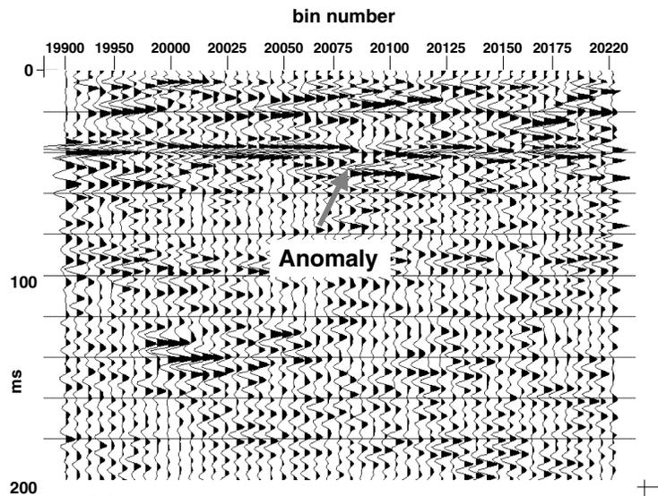
Figure 2. P-S image formed from inline horizontal component of 2000 Chan Chich 3-C seismic survey.
