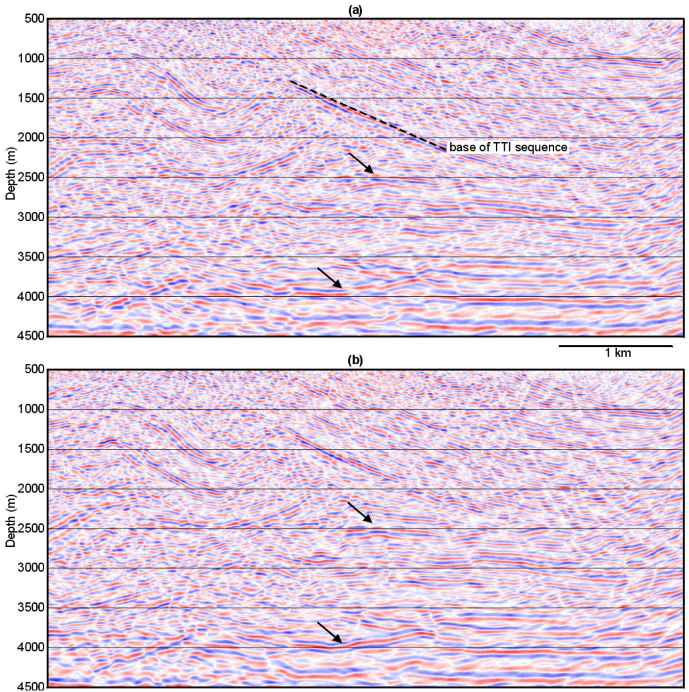
Figure 3. The Alberta Foothills data prestack depth migrated with an isotropic velocity field (a) and an anisotropic velocity field incorporating the TTI parameters derived by inversion (b). The arrows highlight some of the reflectors that are imaged better on the TTI section. The base of the TTI sequence we analysed is indicated.
