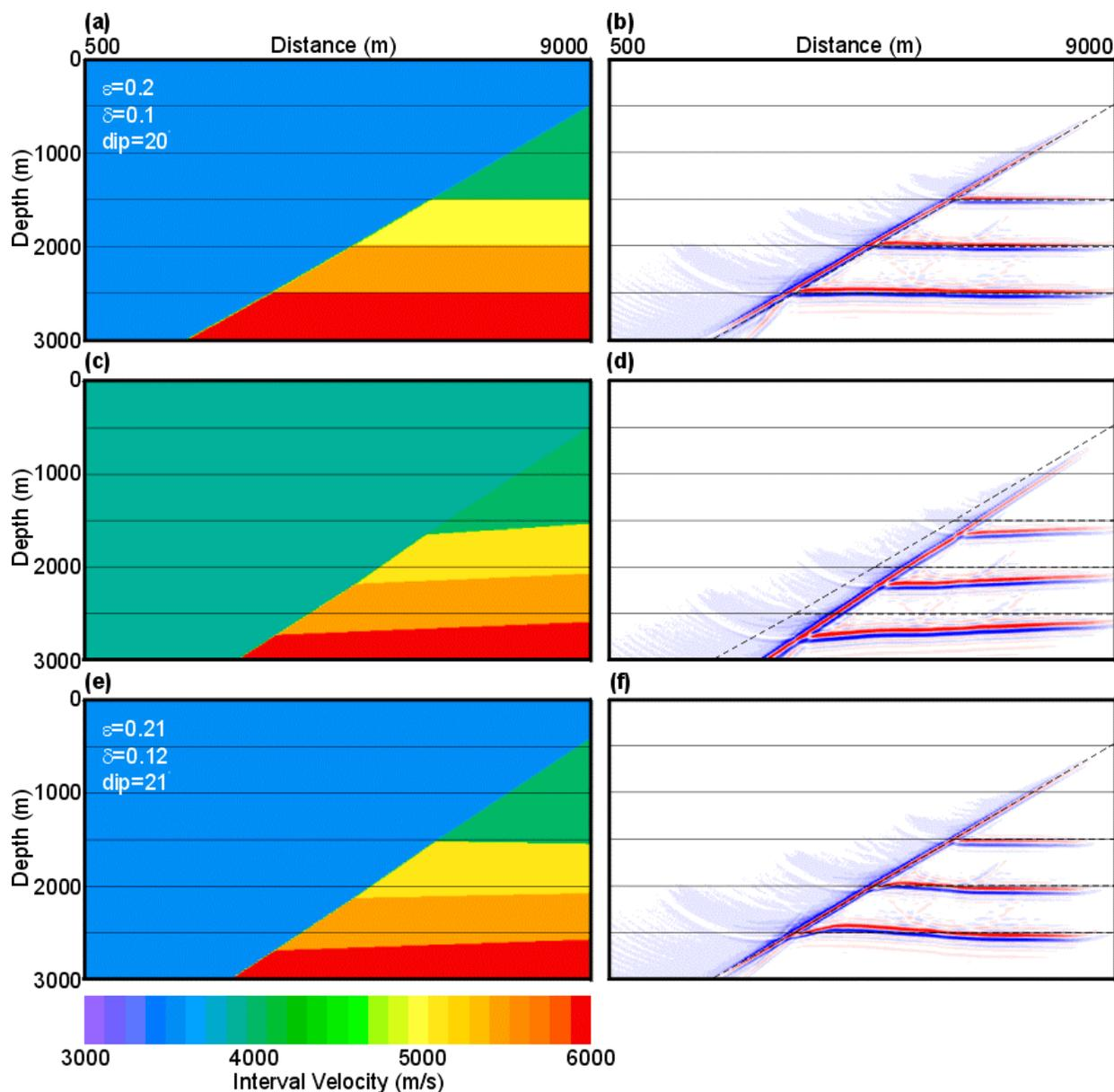
Figure 2. The velocity models (a, c, e) and corresponding prestack depth migrated numerical modelling data (b, d, f). Velocity model (a) is the exact TTI model, (c) is the isotropic model derived through depth velocity model building and (e) is the model of (c) but with the TTI parameters derived by inversion applied to the TTI layer. The dashed lines on the sections indicate the true positions of the reflectors.
