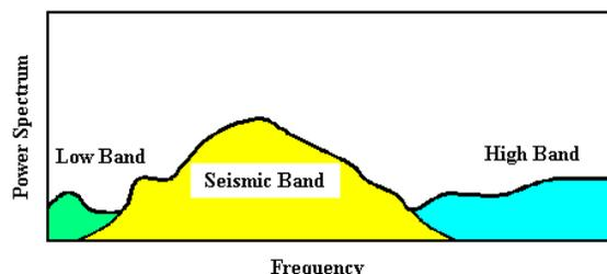
Figure 1. The frequency spectrum of the earth model versus seismic data.
