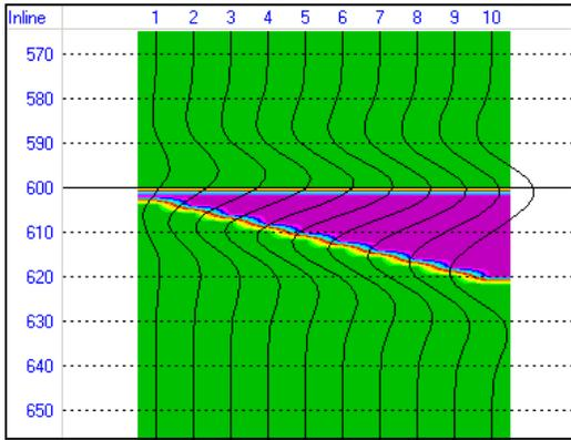
Figure 2. Synthetic traces generated from a wedge model.
