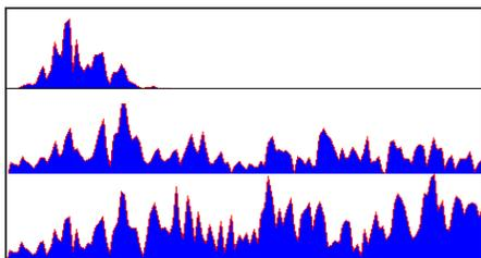
Figure 5. The displays of the power spectrum of the original data (top), that of the reflectivity of the inverted model (middle) and of the true model (bottom).
