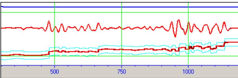
Figure 7. The top curve shows the error between the input and the synthetic. The red middle curve displays the synthetic overlap with the input (black). The bottom curve shows the true model (black) and the inverted model (red).
