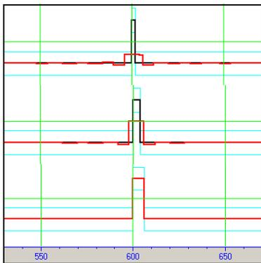
Figure 4. A close look at the inversion result near the resolution limit. The black line shows the true model, the red shows the inverted.
