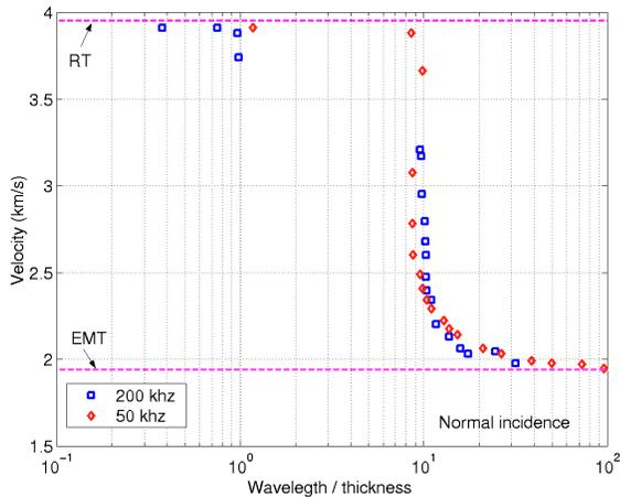
Figure 4. Theoretical scattered P wave velocities calculated from first arrivals as a function of the ratio of wavelength to layer spacing,  $R = \lambda/d$  for normal incidence.
