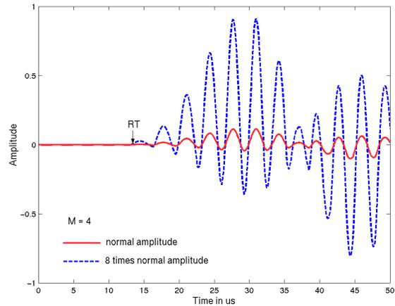
Figure 3. Theoretical waveforms for the plastic/steel stack with  $M = 4$  ( $R = 1.0$ ) at normal incidence illustrating a weak arrival at the predicted ray theoretical time.
