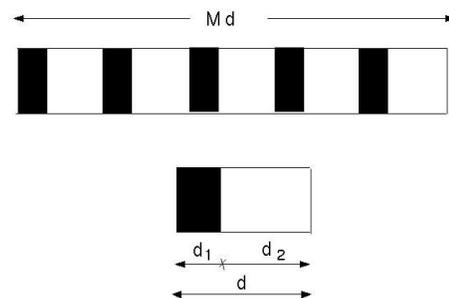
Figure 1. Quasiperiodic structure with two constituent materials. Black boxes represent plastic while white boxes represent steel.
