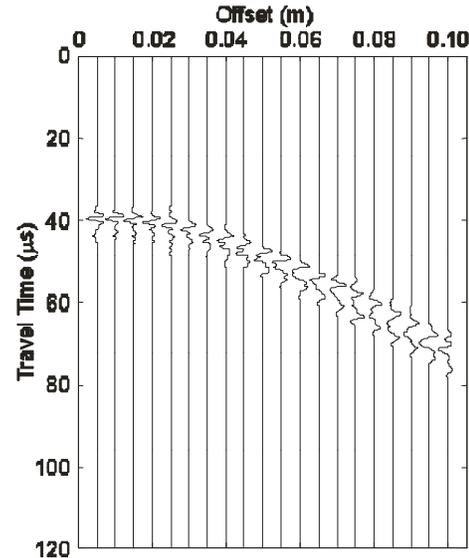
Figure 4. Observed waveforms in Plane 5 from a shear wave source at 4.0 cm depth where the particle motions of the shear waves are predominantly aligned parallel to the sagittal plane.
