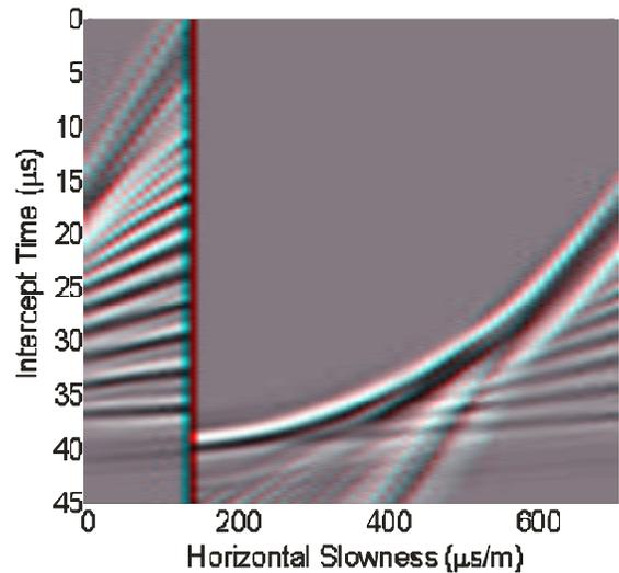
Figure 5. Corresponding  $\tau$ - $p$  transform of Figure 4.
