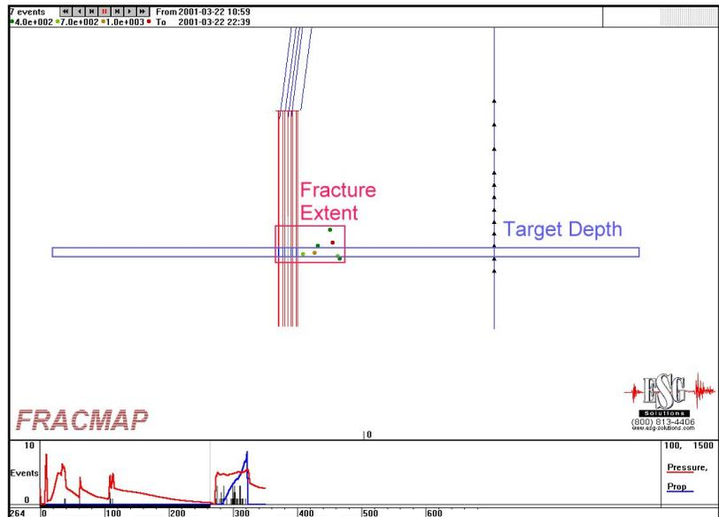
**Figure 1. Longitudinal view of the hydraulic fracture image, showing frac well in red, monitoring well in blue, and geophone locations as black triangles. Events recorded at start of frac are colour coded by injection pressure.**
