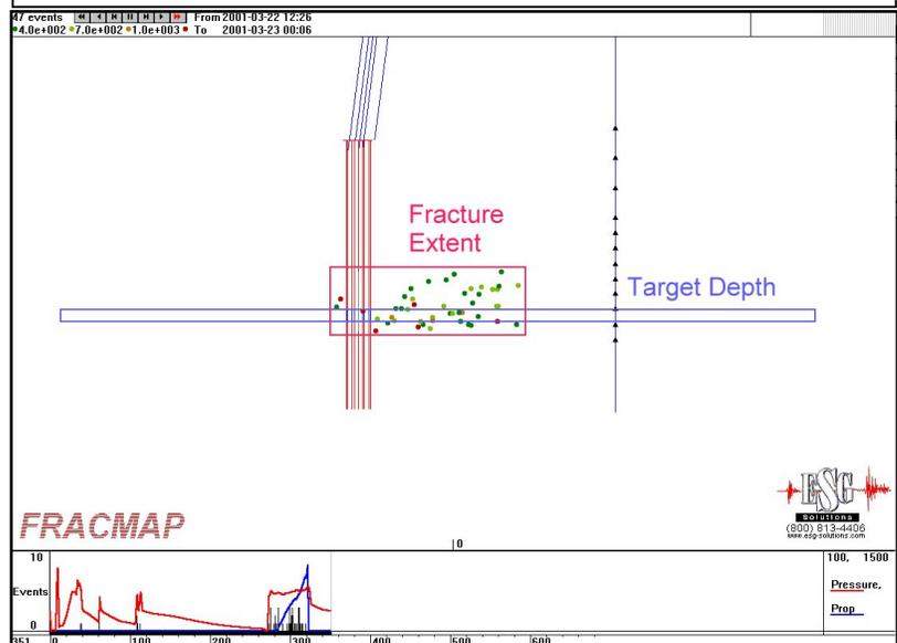
**Figure 2. Longitudinal view of events recorded to the end of the frac.**
