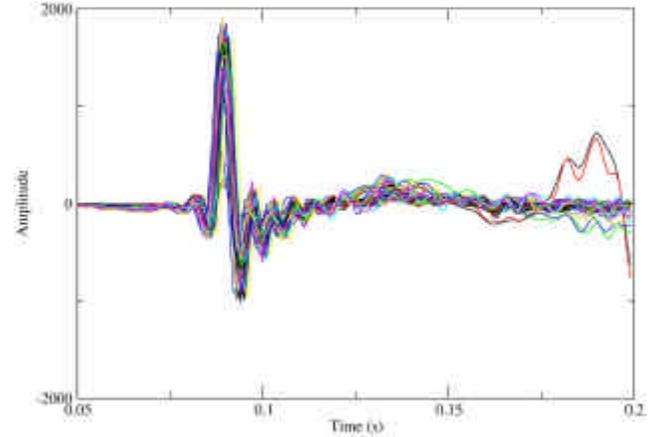
Figure 8: Downgoing wavelets after predictive vibroseis deconvolution in the frequency domain.
