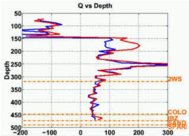
Figure 6: Q versus Depth calculated from VSP survey. Calculation was done using geophones of 90 m. separation.
