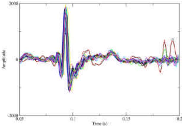
Figure 7: Downgoing wavelets after  $-90$  degree phase rotation and zero-phase deconvolution
