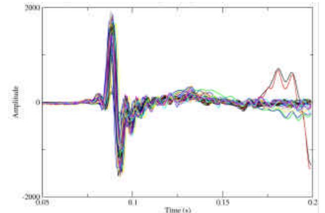
Figure 9: Downgoing wavelets after predictive vibroseis deconvolution with a minimum phase equivalent adjustment for the differentiated Klauer wavelet
