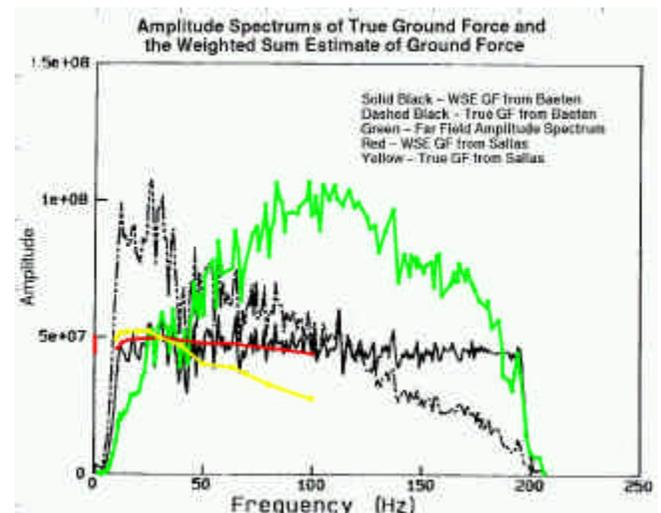
Figure 1: Comparisons of the true ground force and the weighted sum estimate of ground force from Baeten and Sallas
