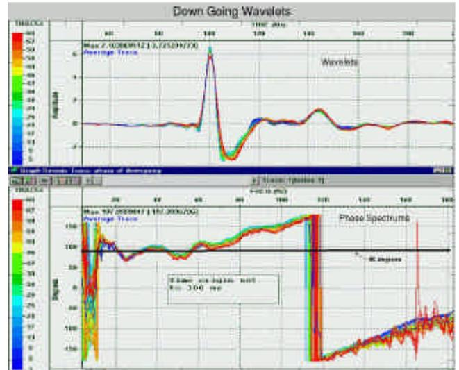
Figure 3: The 66 downgoing wavelets and their phase spectrums after wavefield separation
