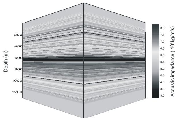
Figure 1: 3D seismic impedance model derived from borehole geophysical logs. The grid spacing is 4m.
