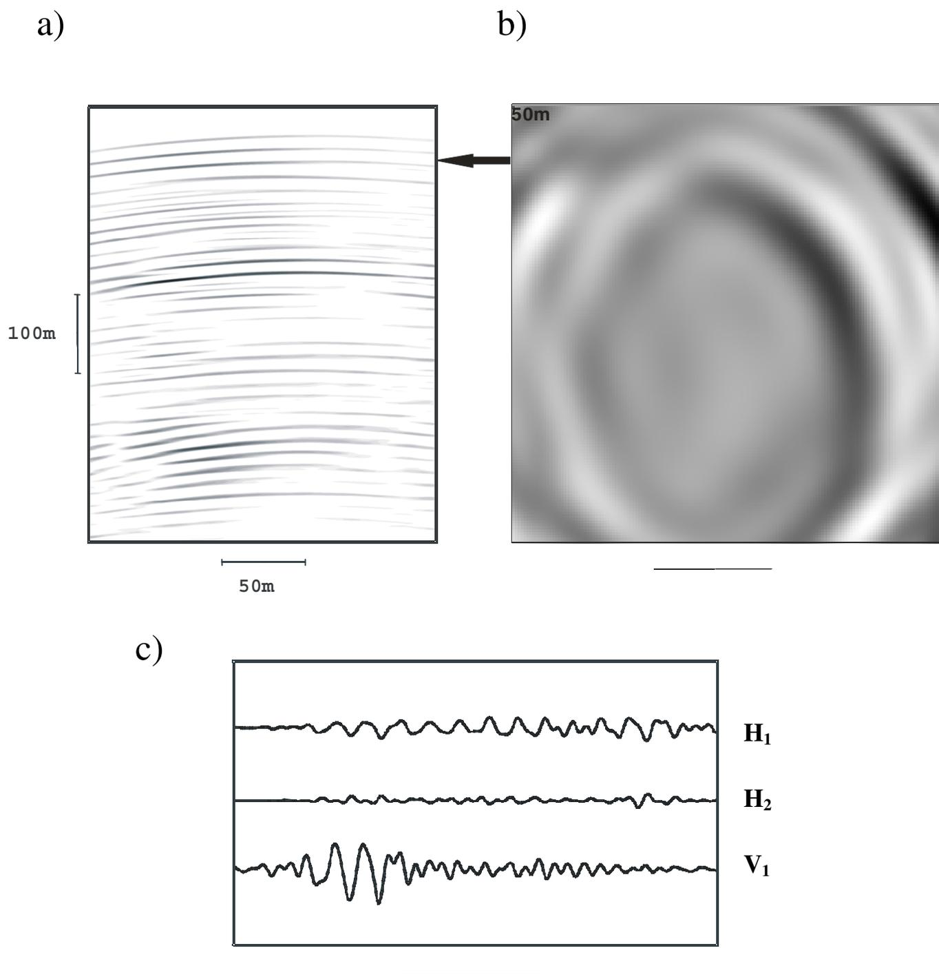
Figure 3: Continuous waveform data recorded with 3-component surface array (a) Snapshot of vertical component in-line section of seismic data excited by the source distribution shown in Fig. 2. Note the pronounced transmission coda trailing the direct event. (b) Time slice through synthetic surface array data with seismic event identified by circular amplitude event centered above the source location. (c) Three-component seismic data example with transmission coda.
