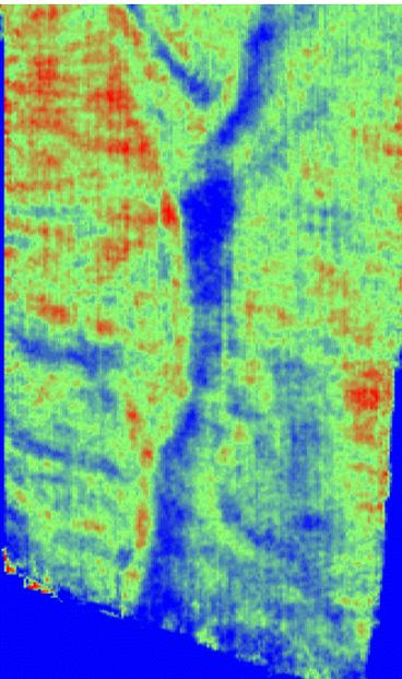
Figure4a: time slice on the rms amplitude stack with the manual velocity picking.
