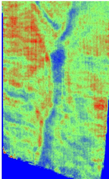
Figure4b: time slice on the rms amplitude stack with the filtered velocity field using a median filter.
