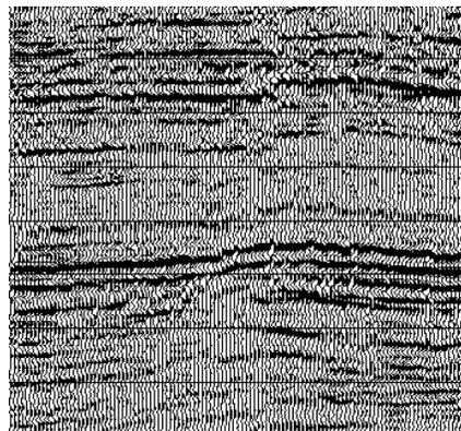
Figure 2b: stack section with raw dense automatic velocity field.
