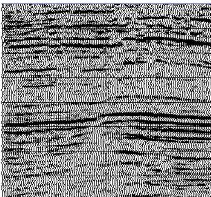
Figure 2a: stack section with manual velocity field.
