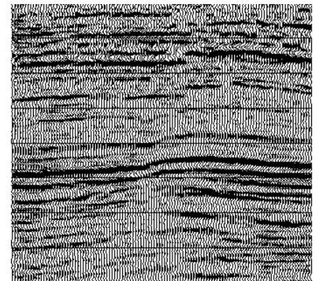
Figure 2c: stack section with filtered dense automatic velocity field.
