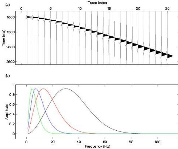
Figure 1: (a) An event in a CMP gather is generated by a reflector in an absorptive medium, where amplitude has been normalised with respect to the maximum amplitude. (b) Amplitude spectra of the events of the input source signature, trace 1, 11 and 21 respectively from the right to the left.
