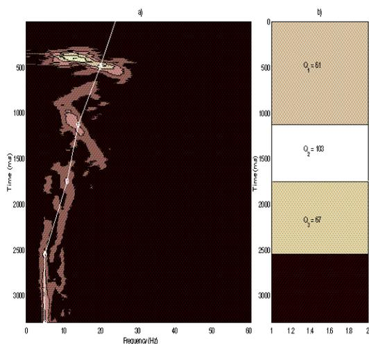
Figure 3: (a) A WTVS of a real seismic trace. The picked peak frequency points are marked by circles and connected by straight lines. (b) the estimated quality factors, the value of the last layer is infinite.
