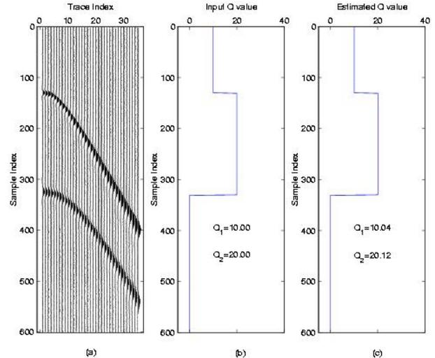
Figure 2: (a) A synthetic CMP gather of two reflections with absorption and 10% random noises, Traces have been normalised based on their maximum amplitude. (b) Values of input quality factors. (c) Computed quality factors.
