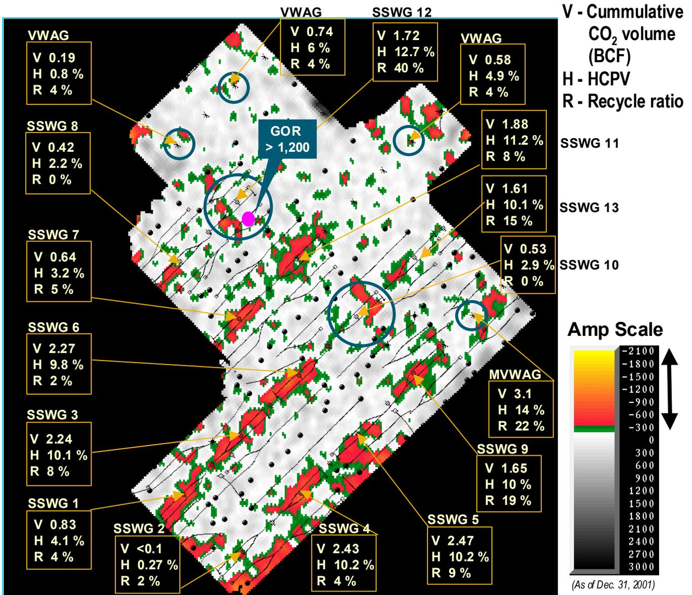
Figure 3 Integrating 4-D monitoring information with production engineering data (cumulative CO<sub>2</sub> injection volumes in billion cubic feet, hydrocarbon pore volume, and CO<sub>2</sub> recycle ratio).
