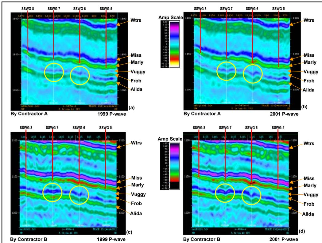
*Fig. 2: A NW-SE 4-D section traversing 4 SSWG patterns. Dual processing yields almost identical results. Baseline (a) and monitor (b) processed by contractor A are compared to corresponding data (c) and (d), respectively, by contractor B.*
