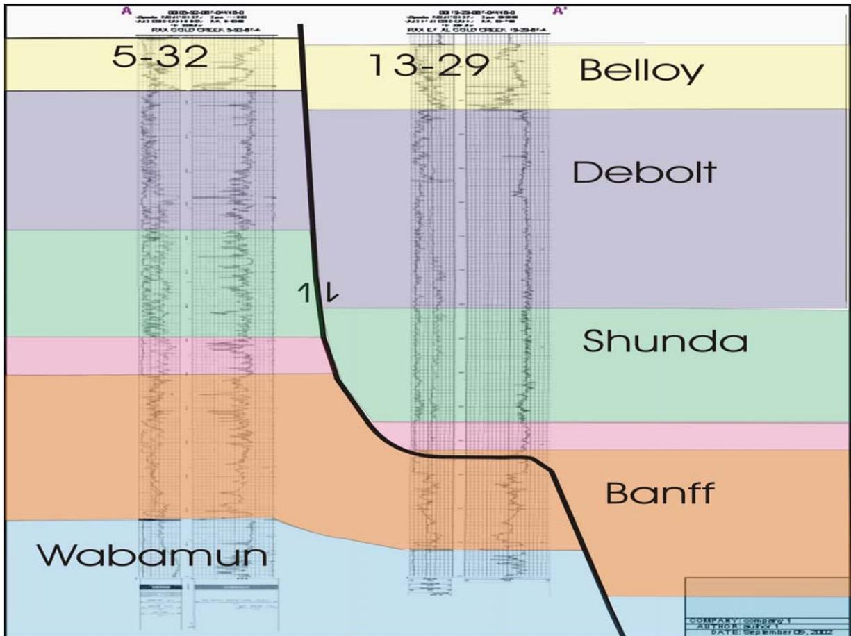
*Fig. 3 illustrates an example of normal faulting along the western margin of the Gold Creek Collapse Structure. Well 13-29-67-4W6 was drilled through a normal fault related to collapse of the underlying Leduc reef. In the hanging wall of the reef, 87m of additional Debolt and 23m of additional Belloy thickness is present, compared to thicknesses at 5-32-67-4W6, only 500m away. The Banff at 13-29-67-4W6 is 67m thinner than at 5-32 because of fault removal.*
