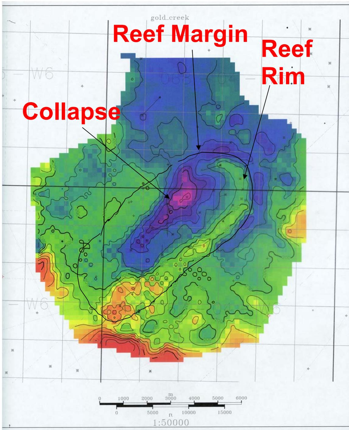
Fig. 2 is a Debolt to Wabamun isochron map. The eastern rim of the underlying Leduc reef appears as an isochron thin. The Gold Creek Collapse Structure immediately to the west of this rim is a NE-SW trending isochron thick. The contour interval is 5 milliseconds and the spectral variation in colour from orange to purple corresponds to increasing isochron values. Figure courtesy of Devon Canada.
