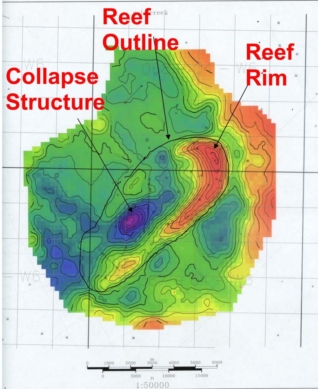
*Fig. 1 is the Wabamun time structure map of the Gold Creek area. Drapes over the eastern margin of the underlying Gold Creek Leduc Reef corresponds to a structural high. The Gold Creek Collapse Structure is a NE-SW trending structural low that is west of the reef rim. The contour interval is 5 milliseconds and the spectral variation in colour from orange to purple corresponds to increasing time structure values. Figure courtesy of Devon Canada.*
