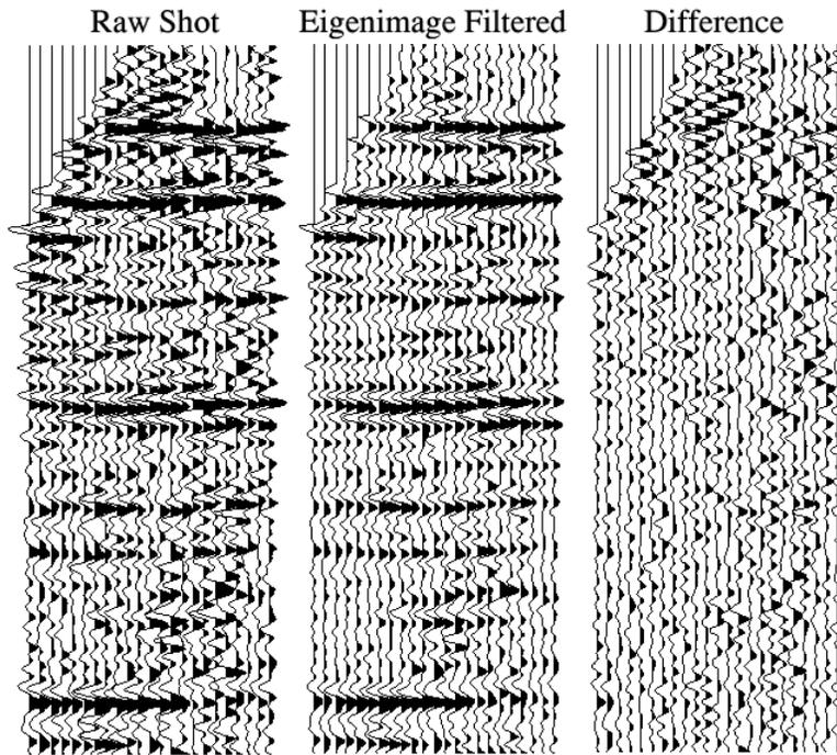
*Fig. 4: A single 24-trace shot record before and after eigenimage filtering of the entire line.*
