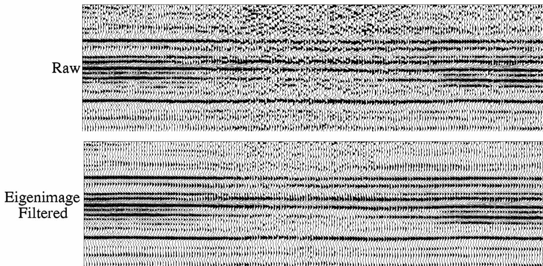
*Fig. 6: An inline slice through a stacked 3-D volume, without and with prestack eigenimage filtering. A rank of 1 was used, which is harsh for all but very flat data.*
