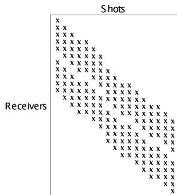
Fig. 2: A surface stacking chart where unstacked traces are positioned according to shot and receiver.
