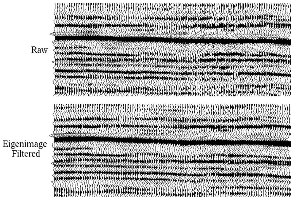
*Fig. 5: Migrated stacks of shots in Fig. 4 without and with eigenimage filtering.*
