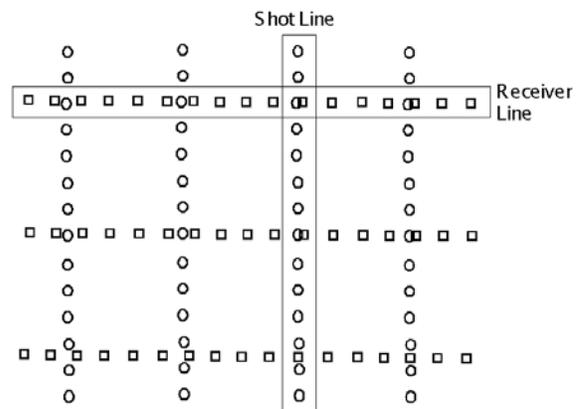
Fig. 3: For 3-D volumes, every combination of shot and receiver line can be filtered separately as if it were a 2-D line.
