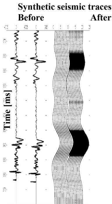
*Fig. 3 The synthetic traces before (gray filling) and after fluid (gray filling) and after fluid replacement (black wiggles) along with the reflectivity time series for both cases.*
