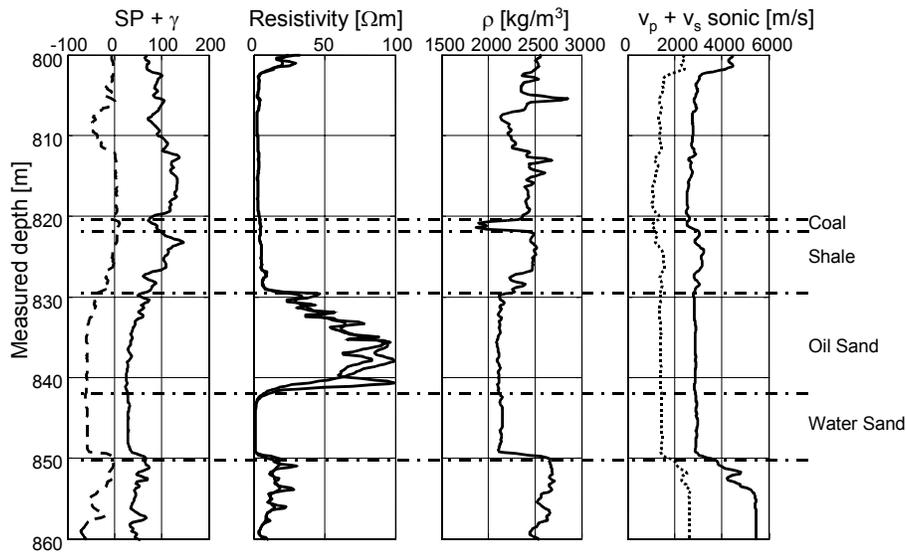
Fig. 2 In the well log the reservoir can be clearly distinguished from the coal and shale layer above and the carbonates below.
