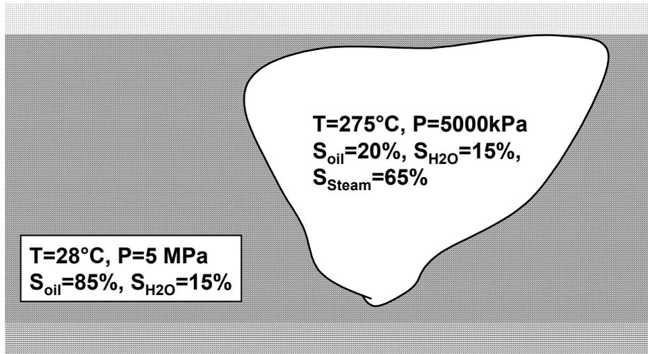
Fig. 1 shows the steam chamber model. Within the steam chamber a homogeneous distribution of the three different pore fluids is assumed.
