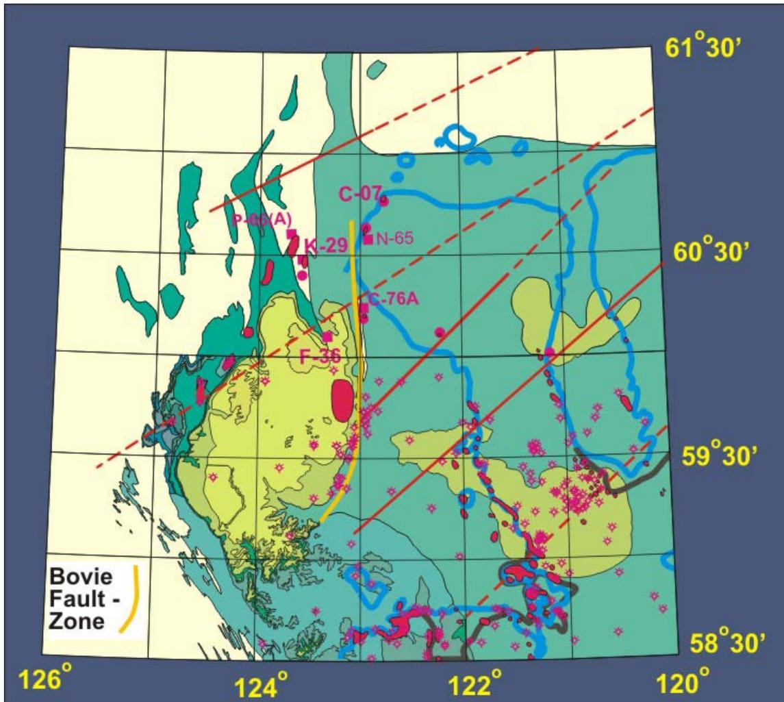
Fig. 1. Map of northeast British Columbia showing Liard Basin west of the Bovie Fault Zone. Cretaceous cover is shown in shades of green. Gas shows, pools and fields are illustrated in red. Also, the northwest limit of the Slave Point (Presqu'île Barrier) is shown.
