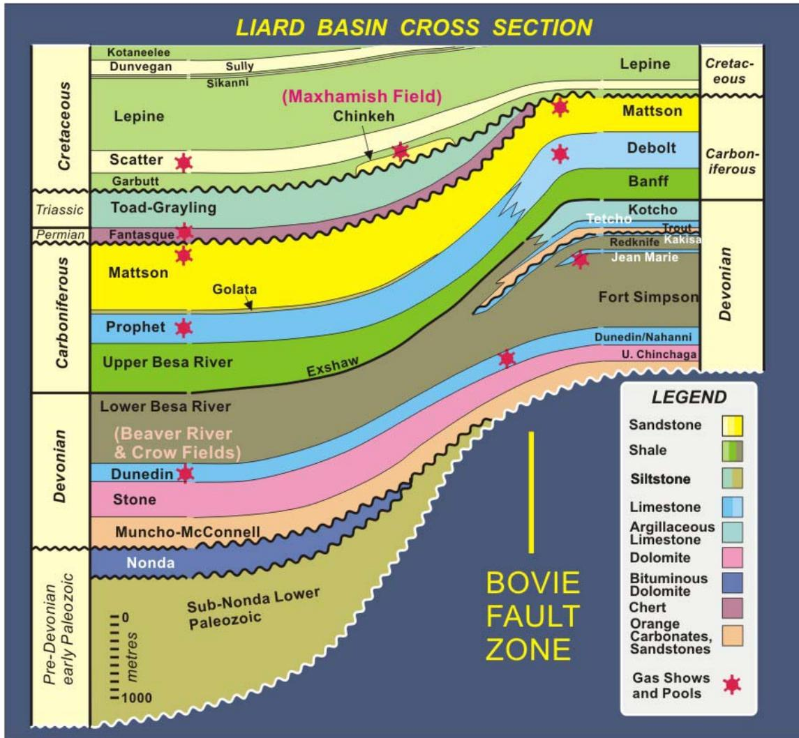
Fig. 2. East-west stratigraphic cross section across the east flank of Liard Basin. Major gas accumulations are shown.
