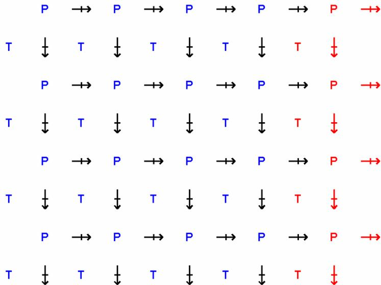
Fig. 2: The right edge of a finite-difference staggered-grid model. The relative position of the x and z displacements (arrows) and P and T scalars are shown.
