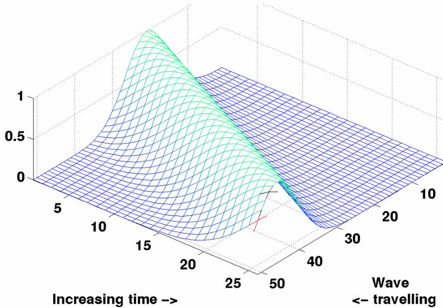
Fig. 1: A surface which represents the time-stepping of a 2D finite-difference model. Stepping within the model (black cross) requires only one equation. Stepping at the edge (red cross) has two unknowns and requires two equations.
