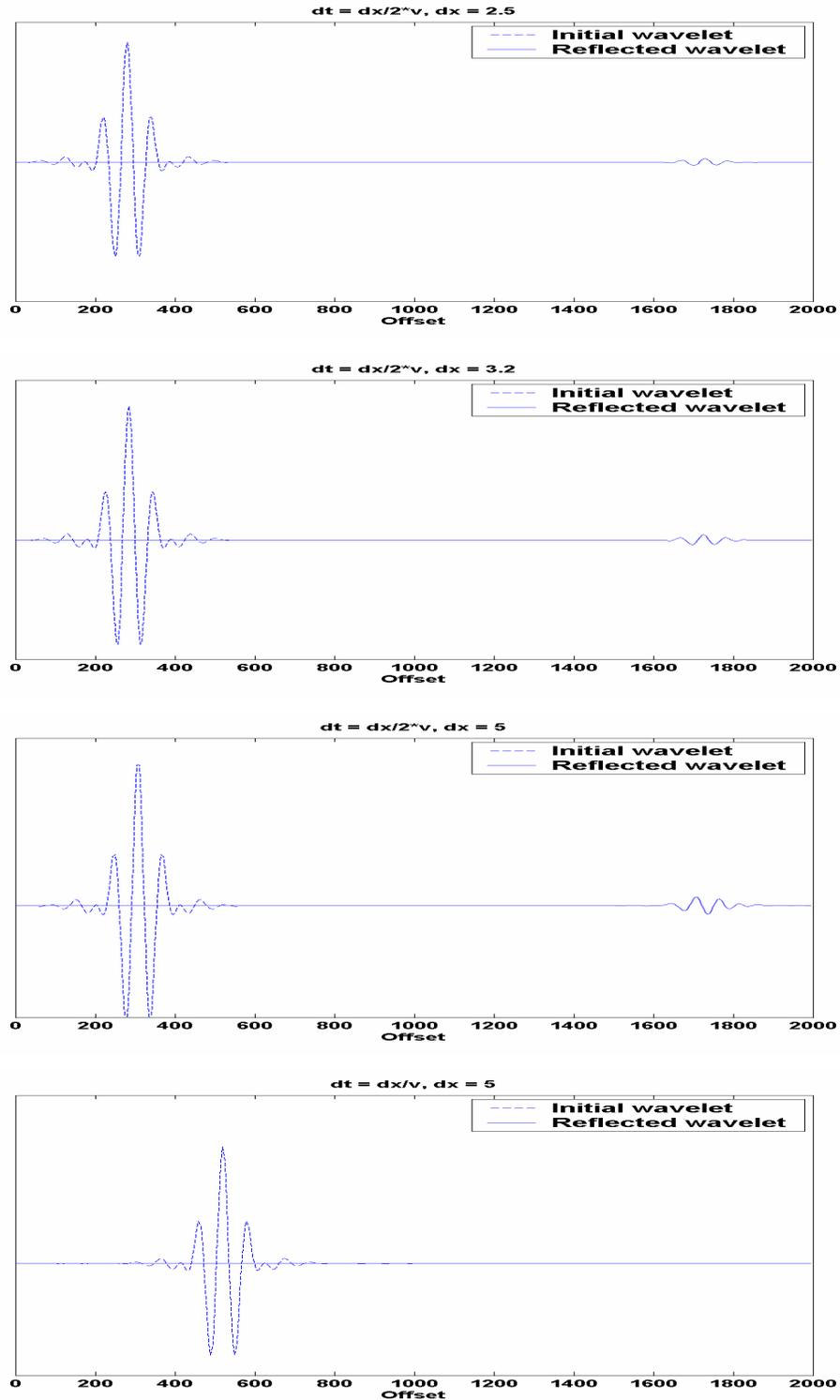
*Fig. 4: The effects of sample rates on a reflection from a transmitting boundary on the right. The upper three graphs show the benefits of the progressively finer sample rates toward the top. The bottom graph shows the complete reflection cancellation under perfect sampling conditions.*
