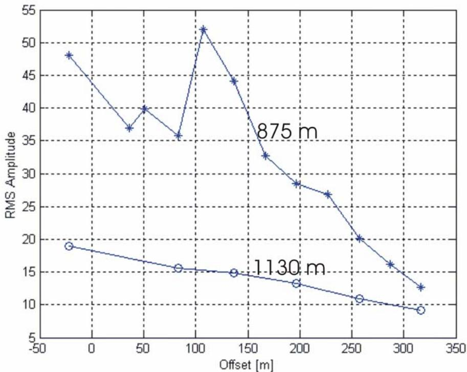
Fig. 5: Field data example of direct (transmitted) arrivals from multi-offset above and below the reservoir zone.
