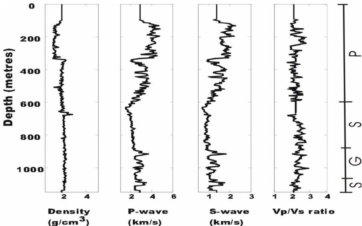
Fig. 2: Acoustic impedance model derived from borehole geophysical logs. P: Permafrost; S: Sediments; G: Gas hydrate
