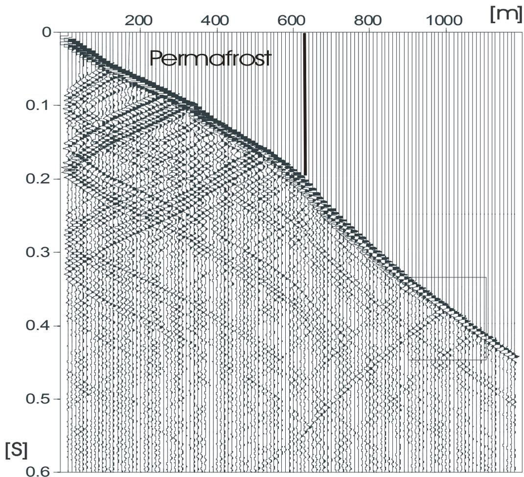
*Fig. 3: Vertical component VSP for the model shown in Fig. 2. The target reflections from the reservoir zone are marked by box.*
