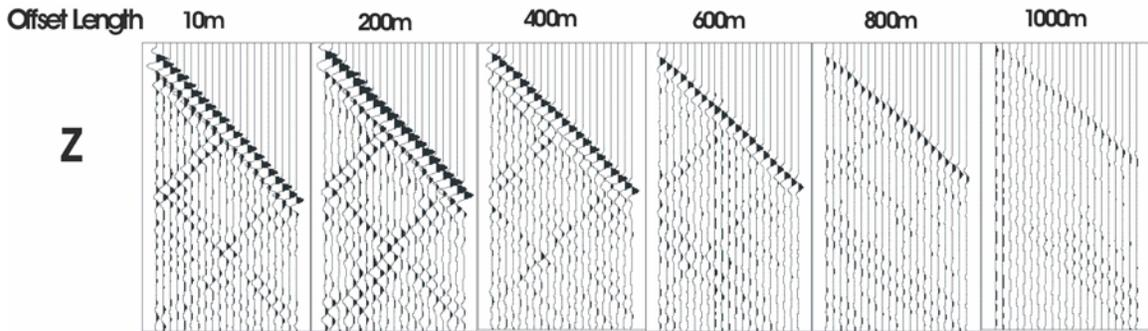
Fig. 4: Synthetic true amplitude recordings (vertical component (top) and horizontal component (bottom)) with reflections from the reservoir for offsets ranging from 0 to 1000m.
