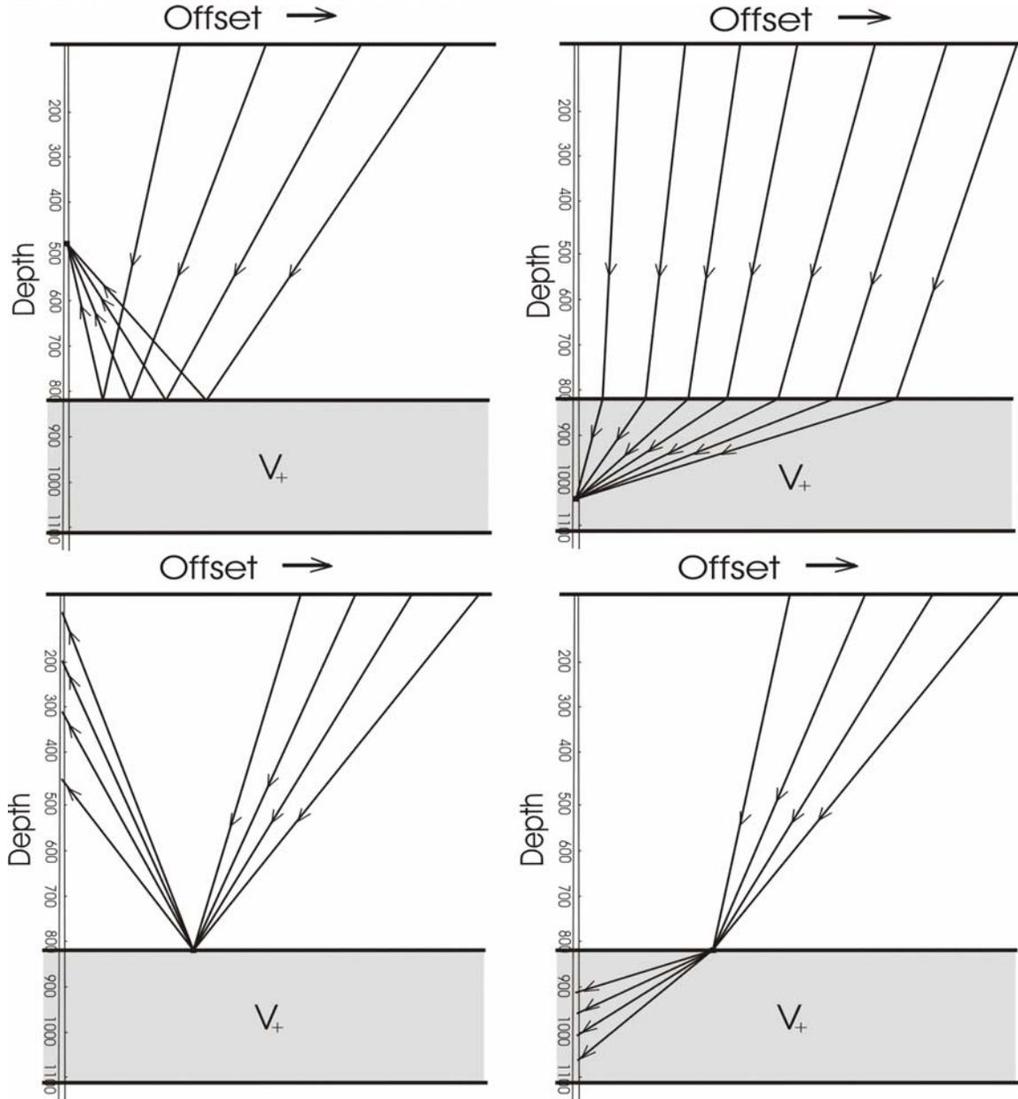
*Fig. 1: Offset VSP data acquisition geometries providing common midpoint and common receiver gathers for reflected and transmitted wavefields.*
