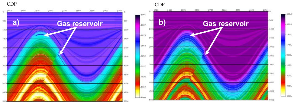
Fig. 2. P- and S-wave velocity for a model with large dip.
