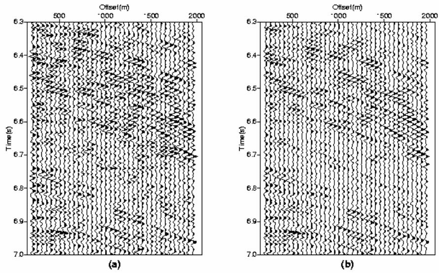
*Fig. 4 - Attenuation of multiples from diffractions. (a) data. (b) data after subtracting diffractions.*
