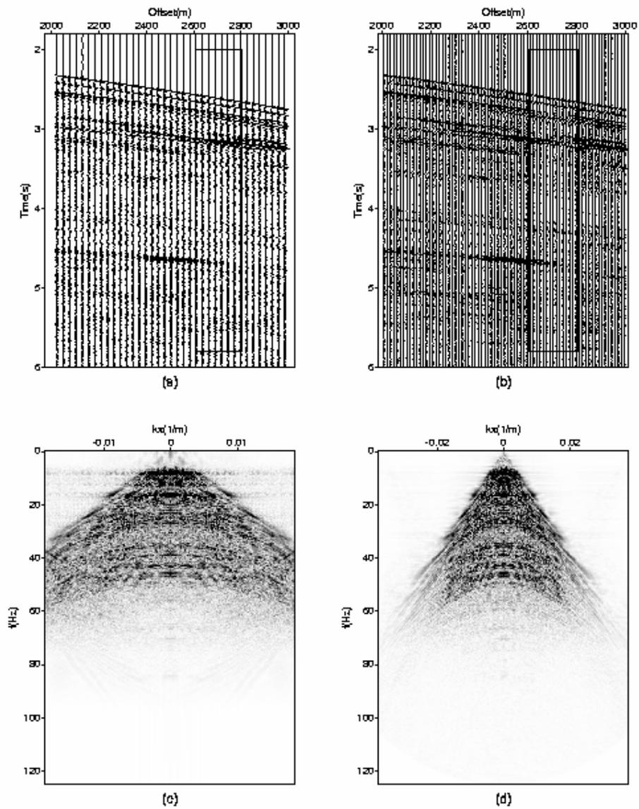
Fig. 2- Gap interpolation and upsampling (a) Shot gather around the far zero offset gap (gap inside de rectangle). (b) Predicted gather with upsampling. (c) FK spectrum of (a), (d) FK spectrum of (b).
