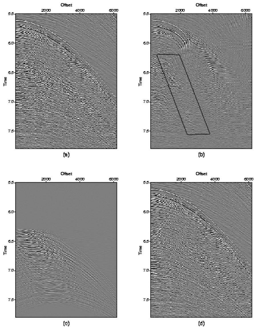
*Fig. 3 - Attenuation of multiples from diffractions. (a) Data. (b) ASRT. (c) Predicted multiples of diffractions. (d) Difference between (a) and (c).*
