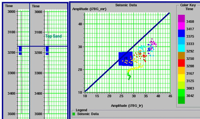
Fig. 11. I-78 LMR crossplot of gas filled sand. The blue polygon correctly identifies the gas filled sand.
