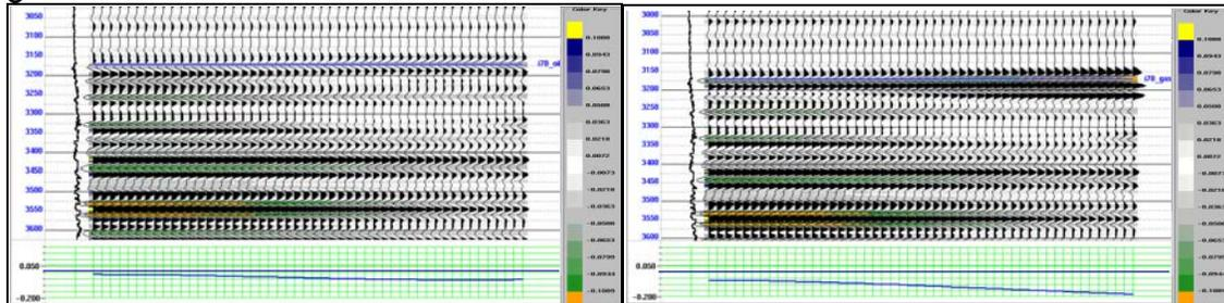
Fig. 6: Oil filled synthetic gather (right) and gas filled synthetic gather (left). The oil gather shows a weak trough at near offsets with a small gradient (Type III). The gas gather shows a strong trough at near offsets with a strong gradient (Type III) .
