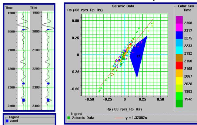
Fig. 8: Rp Rs crossplot of L-08. Points within the blue polygon are highlighted and shown on the Rp Rs traces (left and right respectively).
