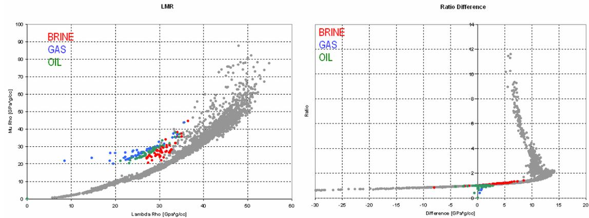
Fig. 4. a) LMR crossplot (left) and b) Ratio-Difference crossplot (right). Note that the LMR crossplot is well constrained in that there are defined relationships between P and S velocities.
