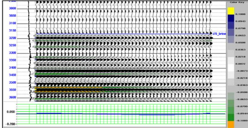
Fig. 5: I-78 brine filled synthetic gather. Amplitude extraction seen in blue.
