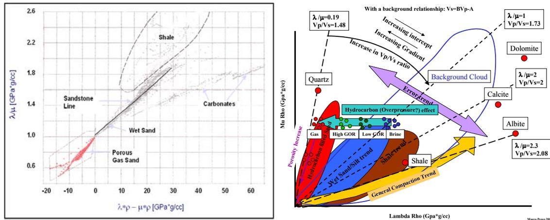
Fig. 2: (a) Ratio Difference crossplot (left) showing fluid and lithology discrimination capability from WCSB well. (b) LMR crossplot (right) with classifications of rocks  $\lambda$  and  $\mu$ : Lamé parameters,  $\rho$ : density (Combination of Goodway, 2001, Downton, 2000).
