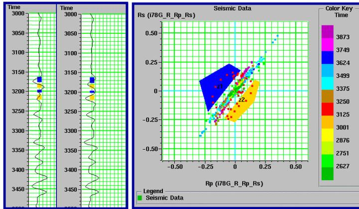
Fig. 9: I-78 Rp Rs crossplot of the gas filled sand. The yellow and blue polygons correspond to the top and bottom of the anomalous zone.
