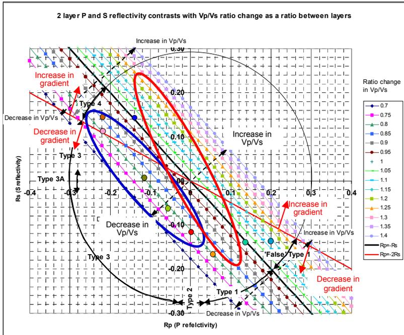
Fig. 1:  $R_p$   $R_s$  crossplot template for AVO type identification (Goodway). Note that the y-axis has been flipped ( $R_s$ ).
