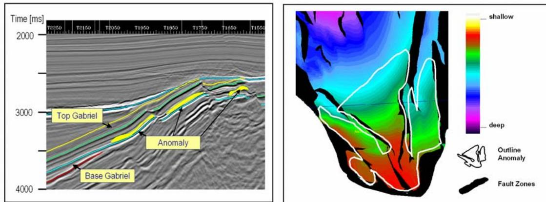
Fig 14. a) Reservoir zone highlighted (left) on Gabriel zone b) Outline of the anomaly superimposed on a time structure map (right)
