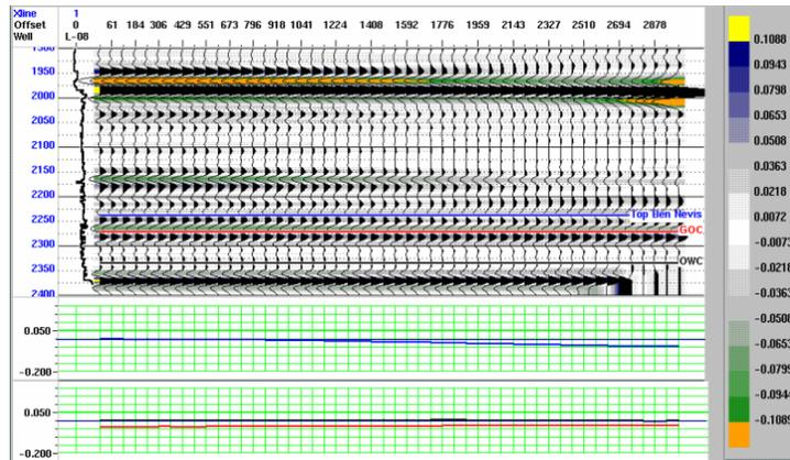
Fig. 7: Synthetic gather created from the L-08 well. The blue pick corresponds to the shale to gas interface, the red pick is the gas to oil interface and the black pick is the oil to water pick.
