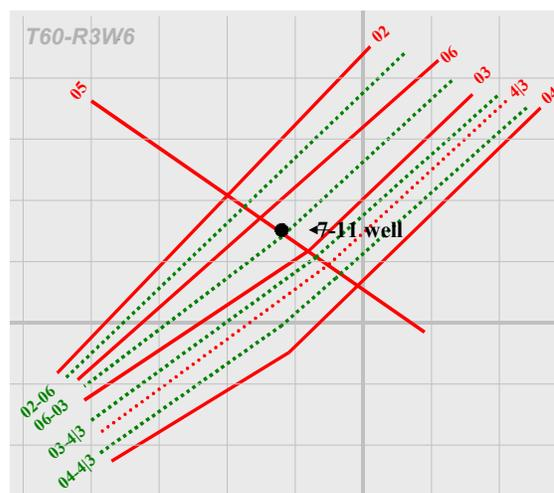
Fig. 3: Acquisition Geometry. Swath data (green) binned into CMP strips between the lines of conventional geometry (red).
