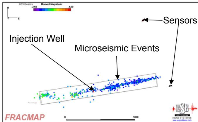
Figure 1: Microseismic events, scaled by moment magnitude, located from acquired waveforms during the hydraulic fracture monitoring project.
