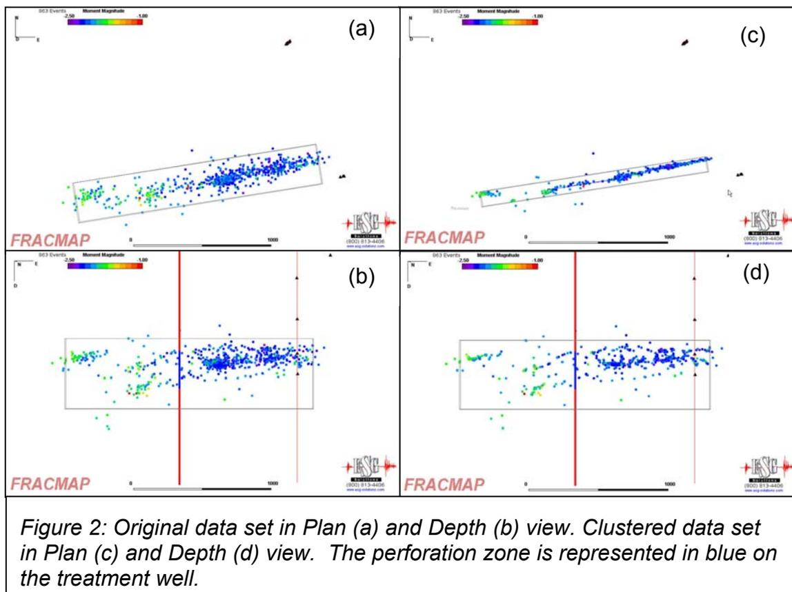
Figure 2 shows a comparison of the original data set (a,b) and the data set after clustering (c,d). The trend of the events is retained and the events define a thin
