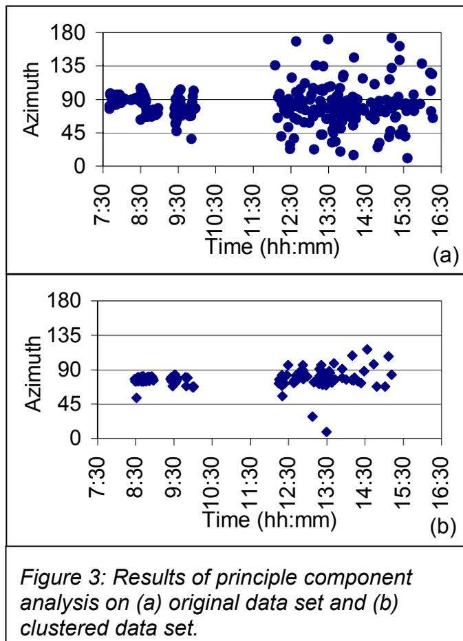
Figure 3: Results of principle component analysis on (a) original data set and (b) clustered data set.
