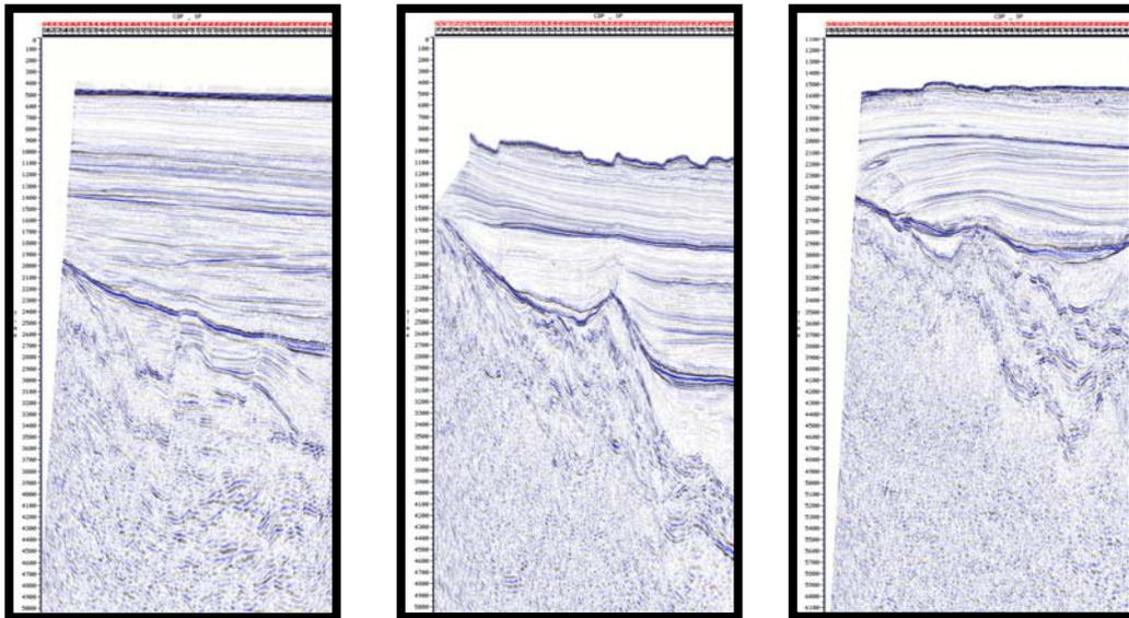
*Fig. 7: Final migrated stacks of test lines after full demultiple application. See fig. 1 for comparison.*
