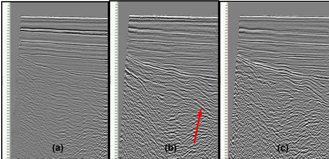
*Fig. 3: (a) Stack of input traces, (b) stacked traces after one pass of Radon demultiple, (c) stacked traces after two passes of Radon demultiple. First pass Radon with conservative velocities removes the water bottom multiple allowing for more accurate velocities and targeting of highlighted peg-leg multiples.*
