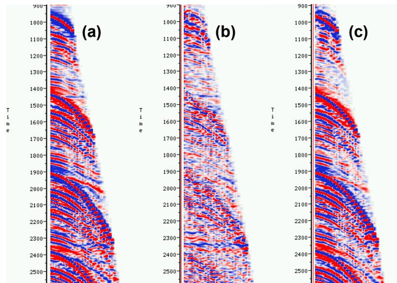
*Fig. 4: (a) Input CMP, (b) input CMP with second order deconvolution operator applied in tau-p domain, and (c) difference between (a) and (b).*
