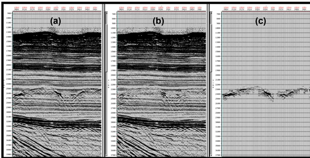
Fig. 6: (a) Input stack with residual dipping water bottom multiples overlain on a flat background, (b) result after application of pattern recognition algorithm, and (c) difference between (a) and (b).
