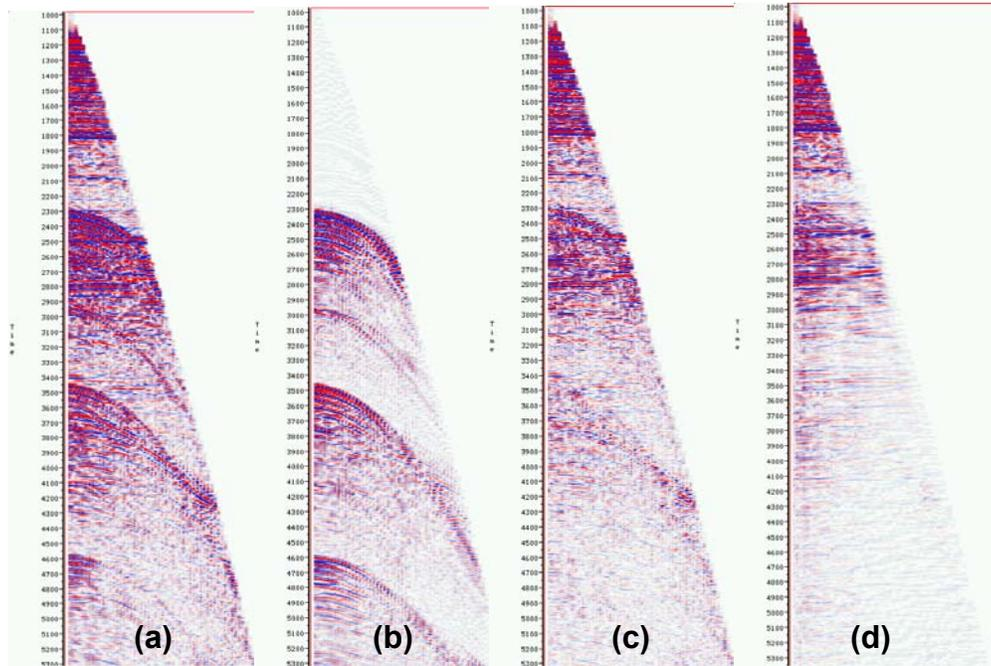
*Fig. 2: (a) Input CMP gather containing 2D and moderate 3D multiple energy, (b) multiple model generated by one iteration of SRME, (c) result of least squares adaptive subtraction of (b) from (a). The high degree of attenuation of the multiple energy found on the near traces represents one of the benefits of SRME techniques. Application of conventional Radon demultiple removes residual multiple energy from the far offsets (d).*
