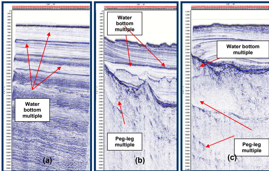
*Fig. 1: Test line stacks from one survey demonstrating varied and severe multiple problems.*
