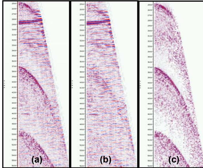
Fig. 5: (a) Input CMP, (b) CMP after frequency separation attenuation, and (c) difference between (a) and (b)
