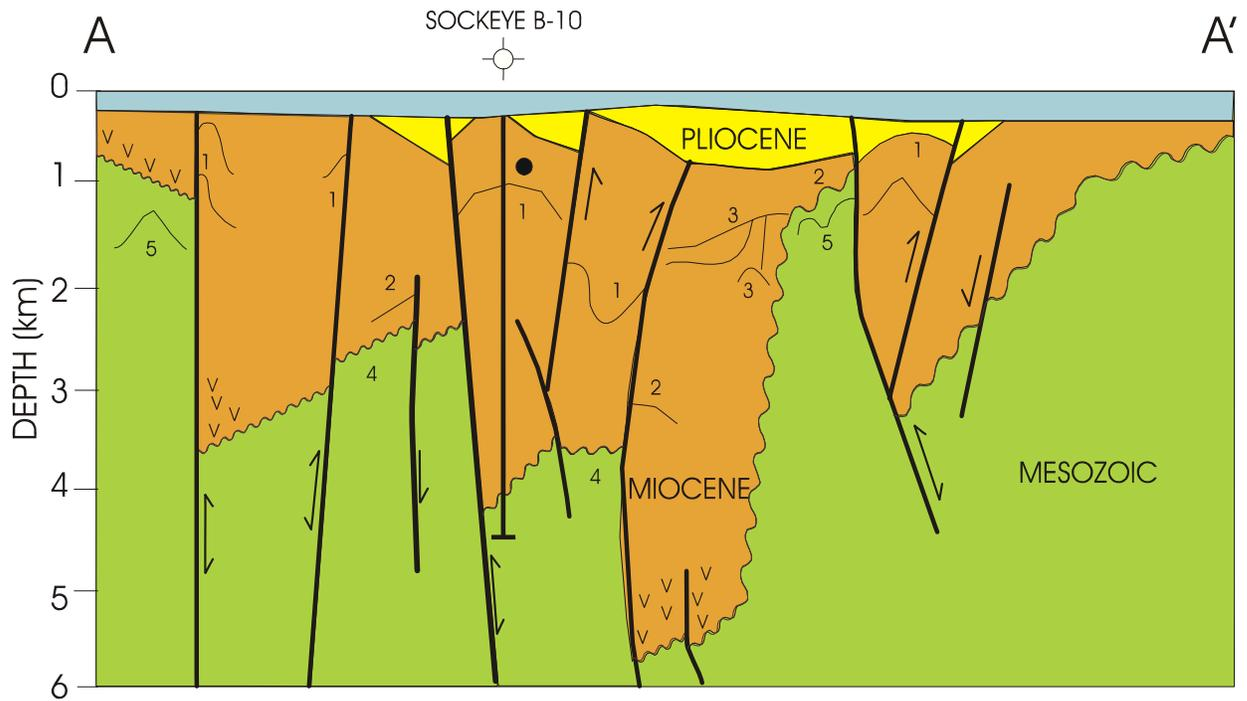
Fig. 4. Simplified structural cross-section for offshore region of Hecate Strait; from Hannigan et al. (1998), modified after Dietrich (1995). Location of line of cross-section shown on Fig. 1.
