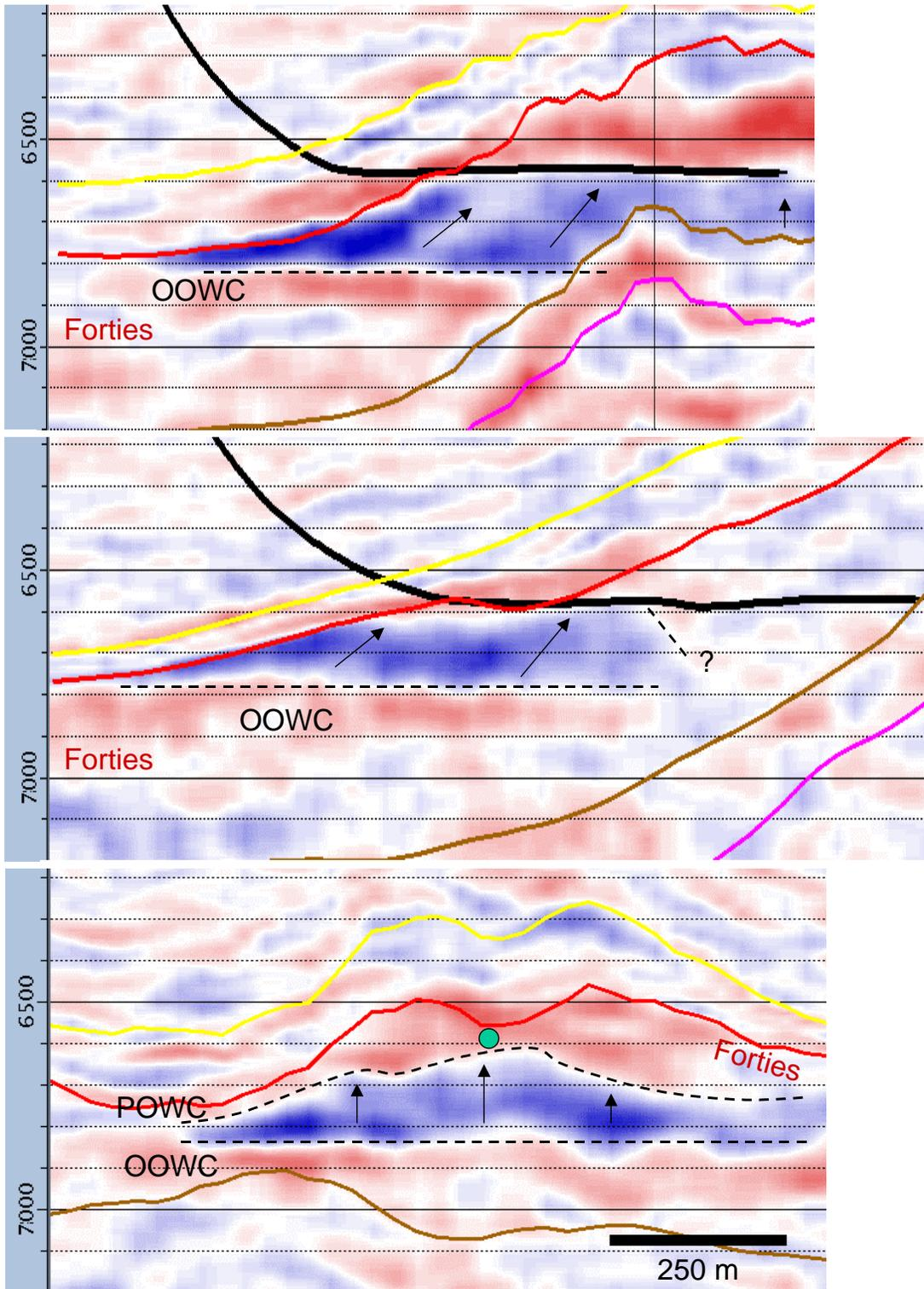
Figure 4. Different flood patterns at well seen on the 98-93 difference cube.
