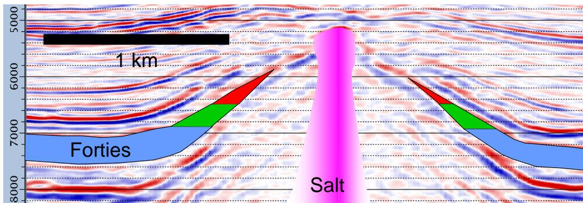
Figure 1. West-east cross section across the northern part of Gannet C showing pre-production fluid distribution in the Forties and very approximate salt structure. All figure depths in ft. (No vertical exaggeration on this figure).
