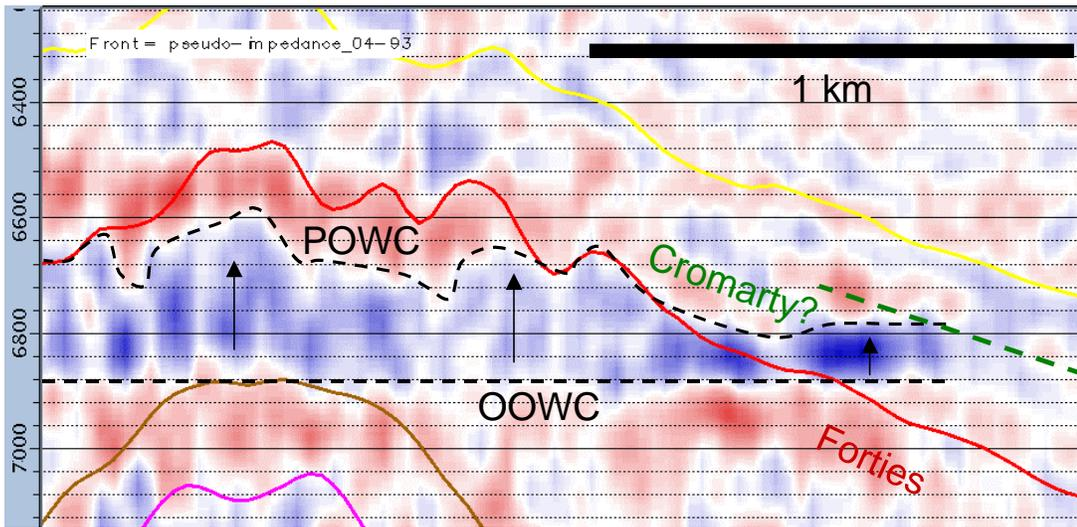
**Figure 6.** In the south-east of the field, (blue) aquifer influx (hardening) extends well outside the top Forties pick on the 2004-1993 difference cube, indicative of significant Cromarty presence, and connection with the Forties. (Note also the highly variable Forties POWC on this section, caused by significant radial faulting orthogonal to section).
