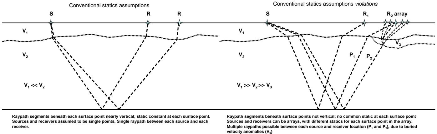
Figure 1. Simplifying assumptions for surface-consistent statics
