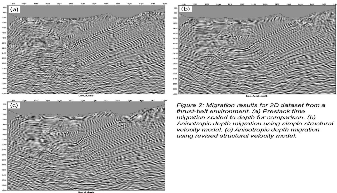
Figure 2: Migration results for 2D dataset from a thrust-belt environment. (a) Prestack time migration scaled to depth for comparison. (b) Anisotropic depth migration using simple structural velocity model. (c) Anisotropic depth migration using revised structural velocity model.
