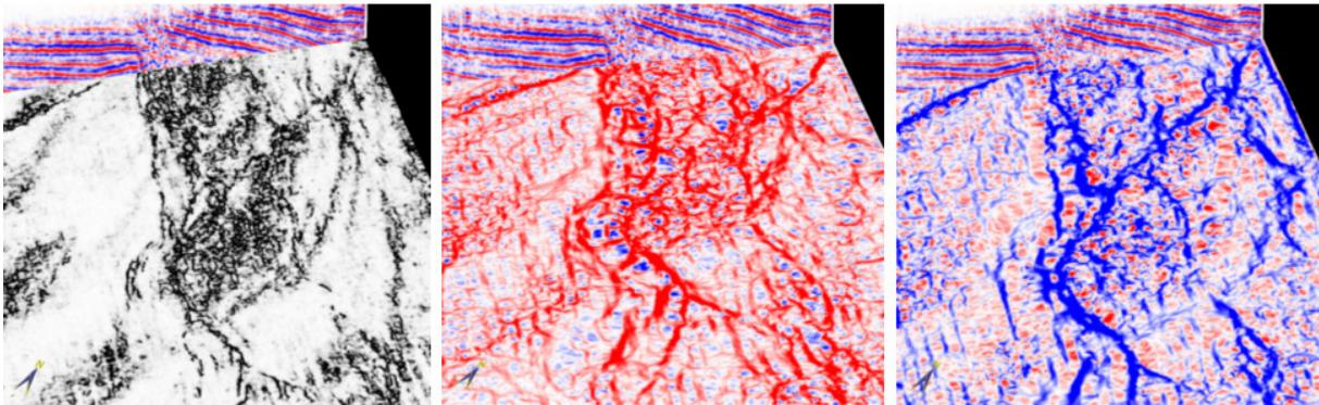
Figure 3: Chair displays showing seismic profiles intersecting (a) coherence, (b) most-positive curvature, and (c) most-negative curvature time slices. Notice the fault/fracture detail seen on the curvature displays is a lot more than seen on the coherence display. (Data courtesy of Rally Energy, Calgary)
