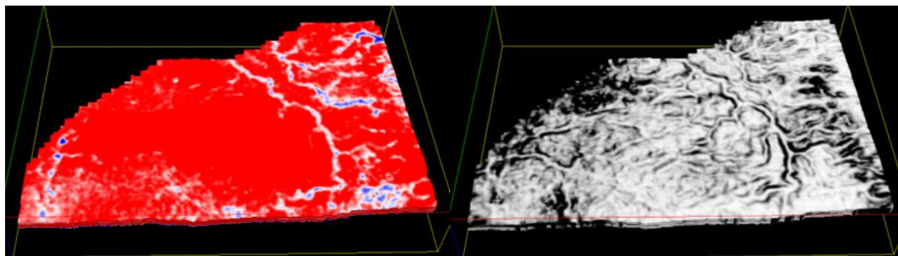
Figure 1: Horizon slices 36 ms below a flattened marker through (a) a seismic data volume from northern Alberta, (b) the computed coherence volume. Notice that as compared with the amplitude slice, the coherence slice very nicely shows the channel system at this level. (*Data courtesy of Arcis Corporation, Calgary*)
