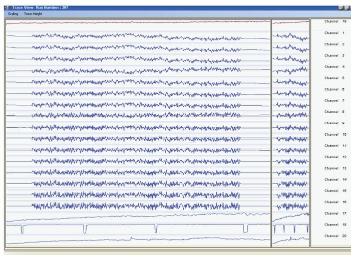
Figure 2: Screen grab from *MTEM Observer*, showing a source record with offset increasing from bottom to top. The response to the PRBS can clearly be seen on all channels. The low-frequency noise level appears to increase from bottom to top, but in reality it is the signal level that is decreasing.
