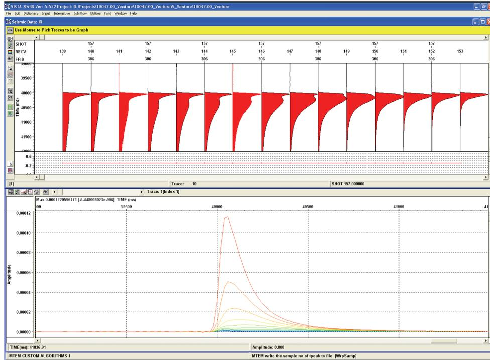
Figure 3: Screen grab from *MTEM QC*, showing recovered impulse responses. In the top display offset is increasing from right to left and the data are normalised to the maximum value. The bottom display shows the same data un-normalised.
