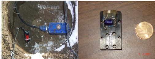
Figure 1: Co-located microphone and 3C geophone (left) in a 30 cm deep hole (right)
