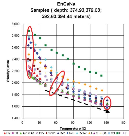
Figure 10: Summarize all (15) the Vp data versus temperature
