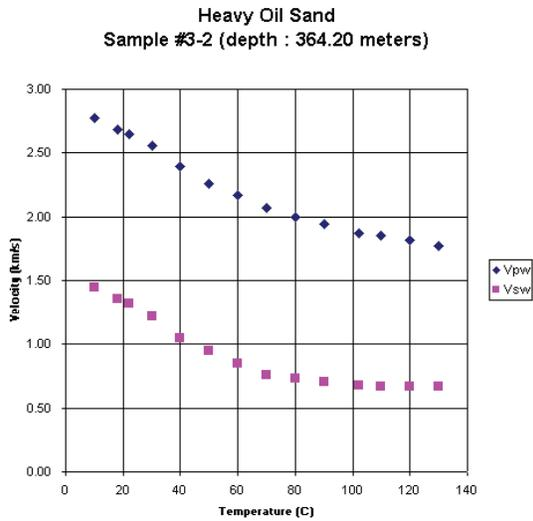
Figure 9: Measure Vp and Vs data versus temperature
