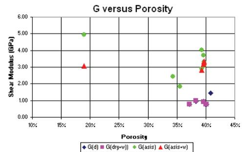
Figure 8: Shear modulus versus porosity
