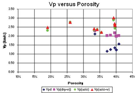
Figure 3: Measure Vp data versus porosity at Pd of 5 MPa.
