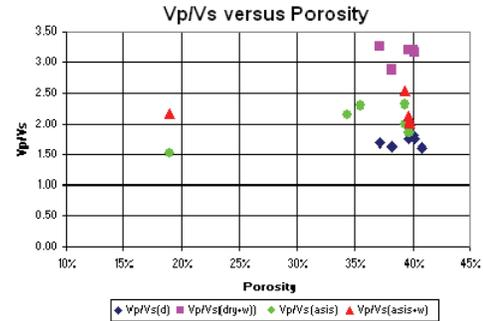
Figure 4: Measure Vp / Vs ratio versus porosity
