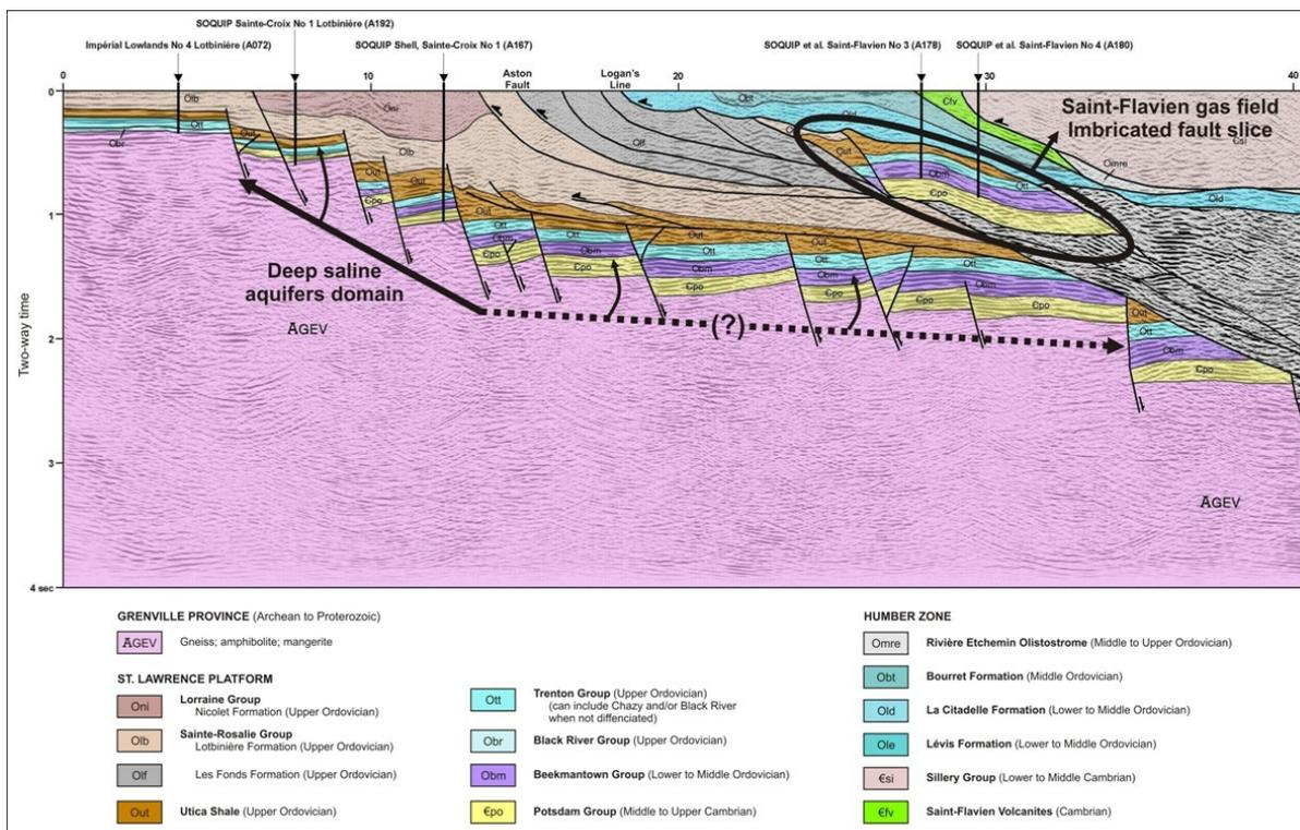
Figure 2: Architecture of the St. Lawrence Lowlands platform and the frontal part of the Appalachian fold-thrust belt, the two domains hosting potential CO<sub>2</sub> storage sites, on seismic line M-2001 (modified from Castonguay *et al.*, 2006).
