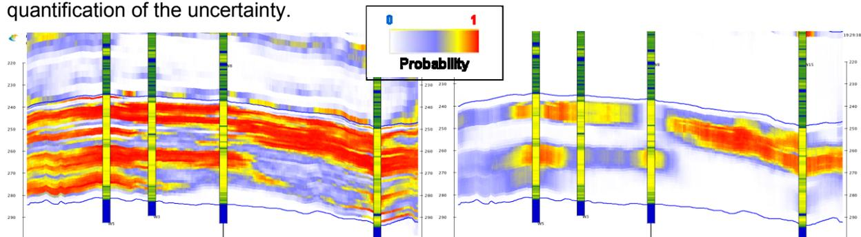
Figure 1: Bitumen probability (left) and thick continuous bitumen probability (right) in a random section (wells coloured by density, sands in yellow, shales in green and carbonates in blue)
