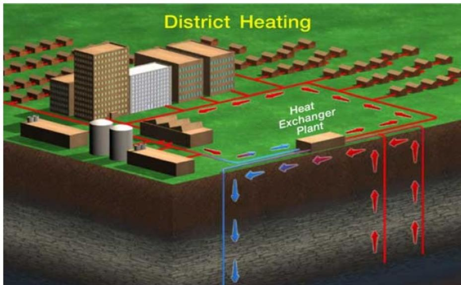
Figure 2 – Model of a District Heating System Triplet Using Geothermal Energy. Figure courtesy the US Geothermal Education Office.
