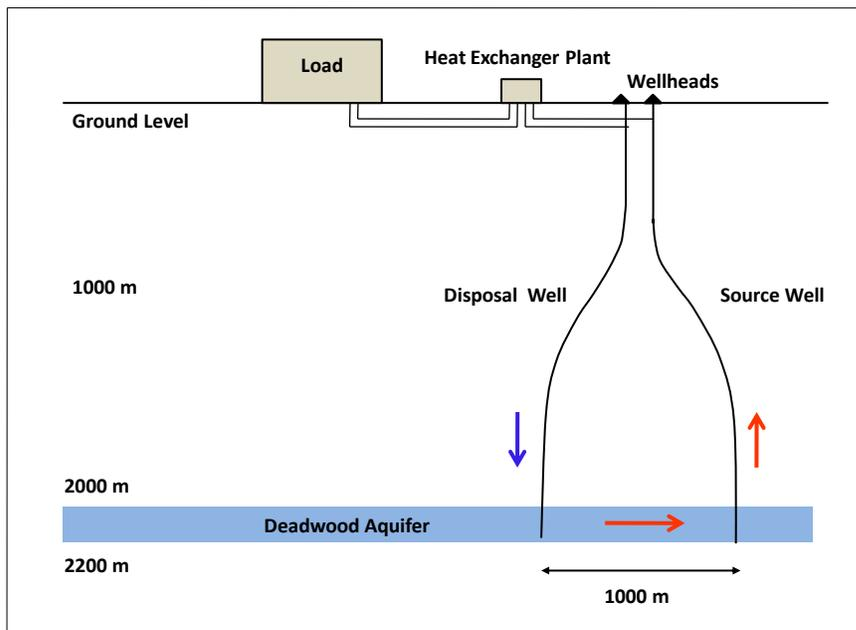
*Figure 1 – Illustration of a model geothermal heating doublet near Regina. The source and disposal wellheads are located close together at surface and the wells have approximately 1000 m separation in the aquifer. The water in the aquifer is relatively stagnant so movement is created by the pumping and injection of the water; arrows show direction of water flow.*
