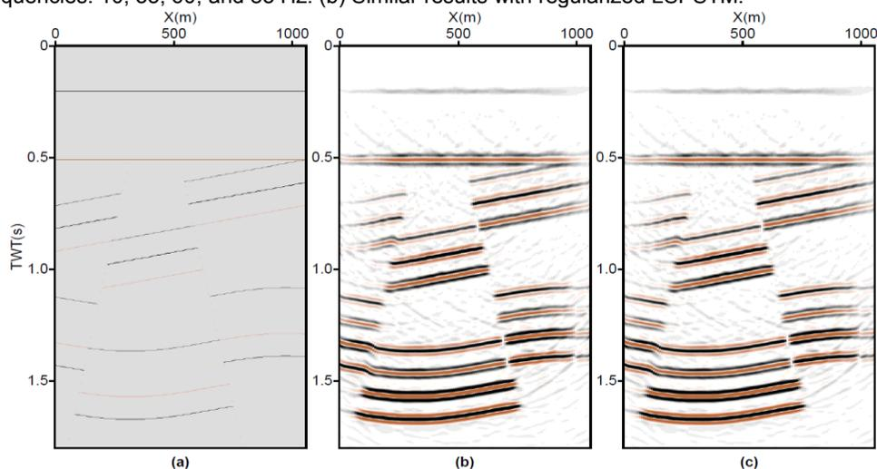
Figure 3. Comparison between true model (a), CGLS (b), and Multigrid CGLS (c) of a synthetic seismic dataset.
