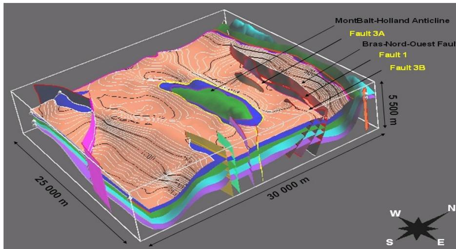
Figure 2: Sectional view of the Gocad surfacic model of the study area in northeastern Gaspé Peninsula with erosion (Eastside view). The first orange surface is the Shiphead Formation, the second blue is the Forillon Formation, the third green is the Chaleurs Group (Saint-Léon Formation), the last two surfaces are unnamed reflectors. Subvertical surfaces are faults identified in the study area. The yellow names are the names of newly identified faults.
