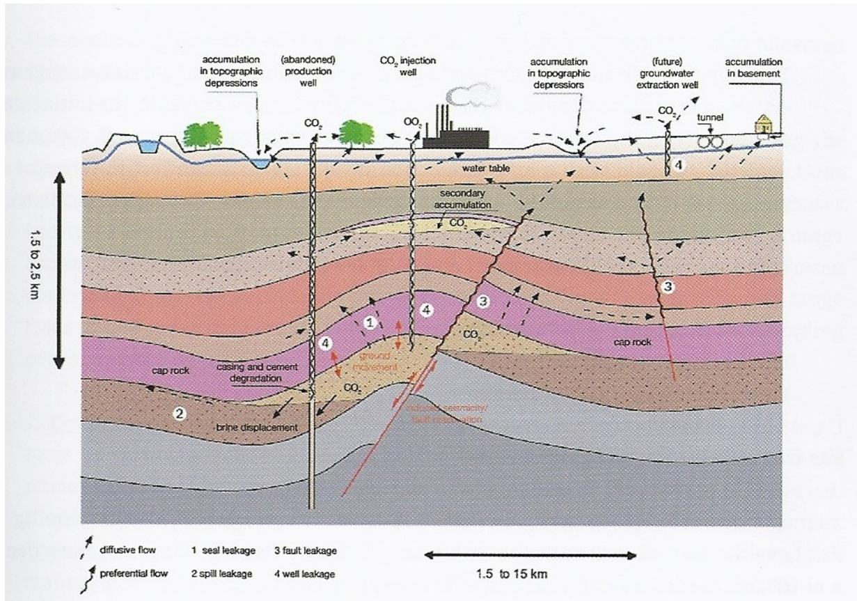
Figure 2: Main leakage paths for CO<sub>2</sub> to move toward the surface: 1) Seal Leakage; 2) Spill Leakage; 3) Fault leakage; 4) Well leakage. From Pagnier, 2009.
