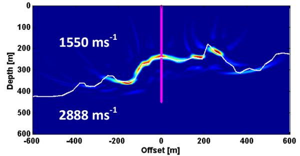
superimposed white line represents the true model contact. The P-wave velocities are for the soft sediments and the breccia unit respectively.
