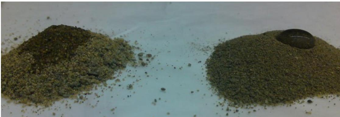
Figure 1: Indication of Wettability Changes: Clean Soil (left), Diesel-Impacted Soil (right)
